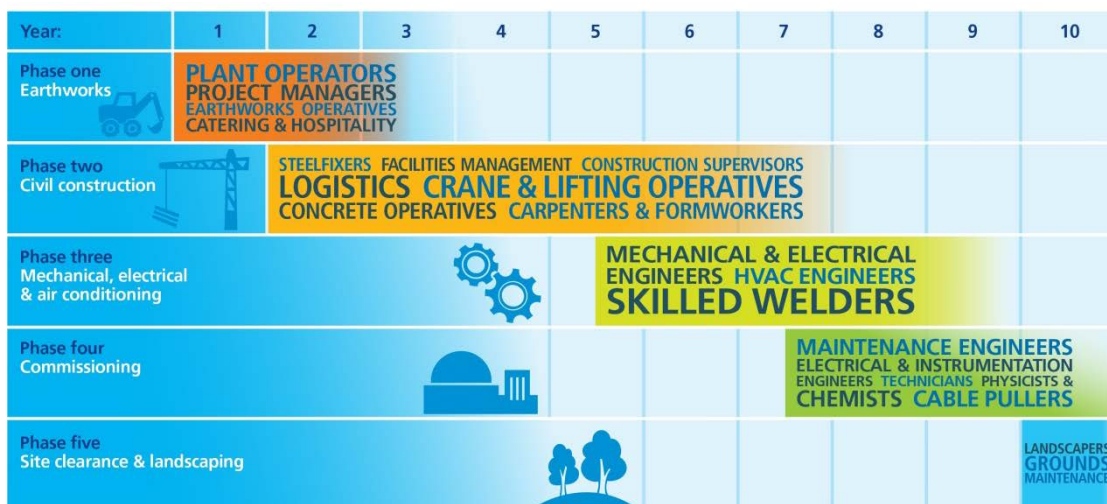
Figure 3: Phases of construction and forecast job types on Hinkley Point C throughout construction (Source: NNB HPC)
