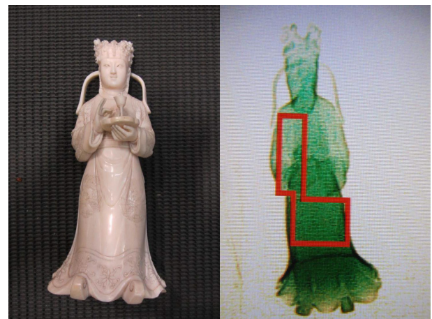
Figure 2: Images of an ivory ornament seized by UK Border Force. X-rays of the seized items indicate whether they contain non-organic materials, which includes ivory among others, and are shown by the areas of green.
