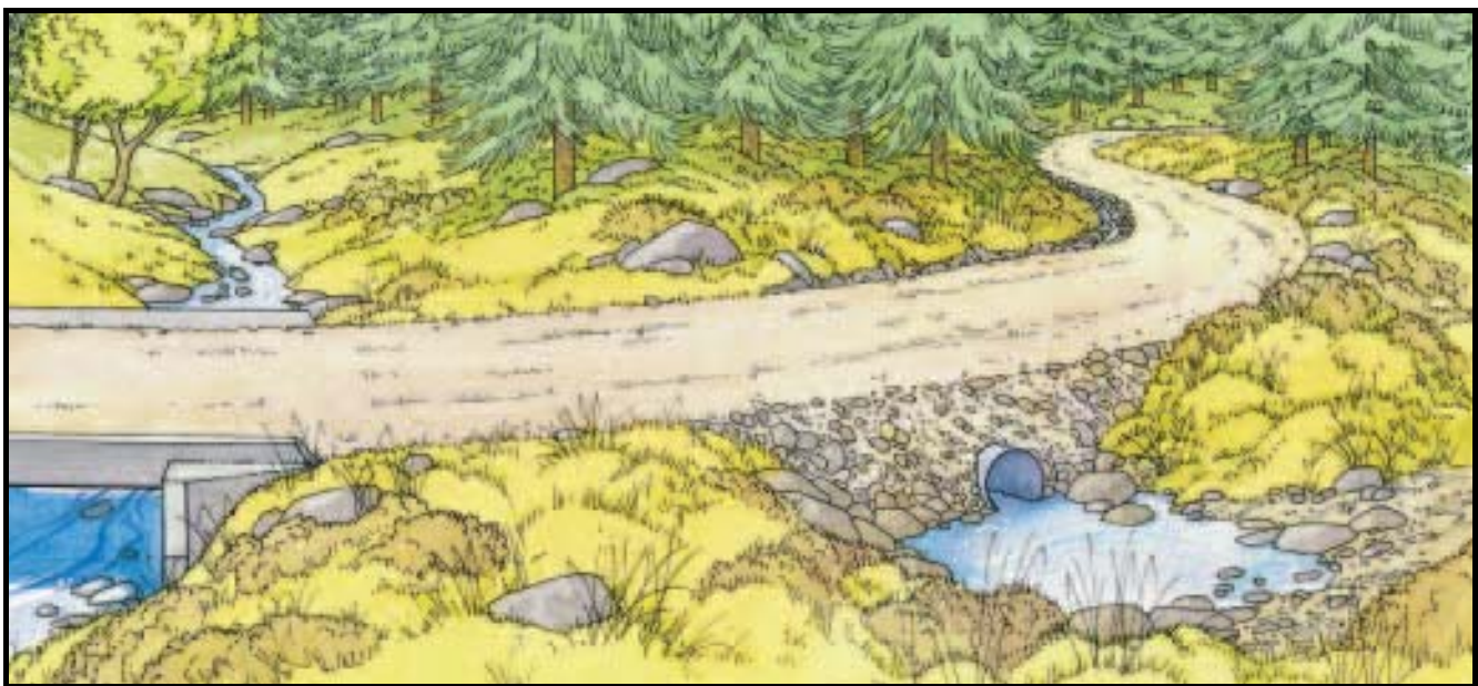
Figure 6: A cut off culvert
