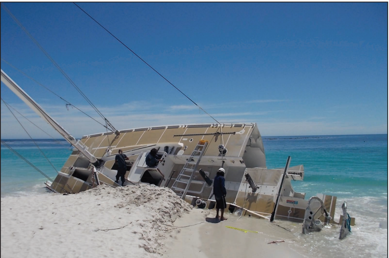
Figure 6: Disposal of CV24 by cutting into sections and removal from the beach
