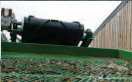
Screening wood chip to improve chip quality
