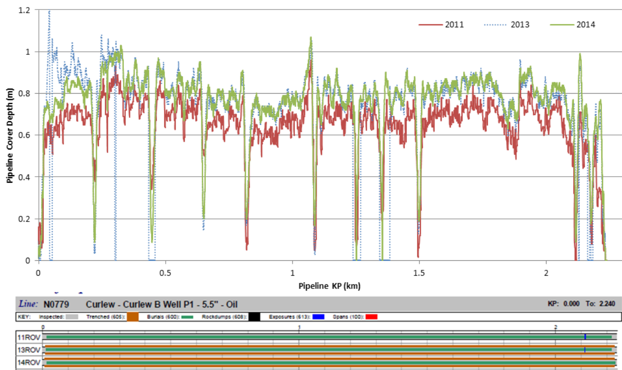
Figure 8-2 – Curlew B Production Pipeline Cover Depth Survey Data
