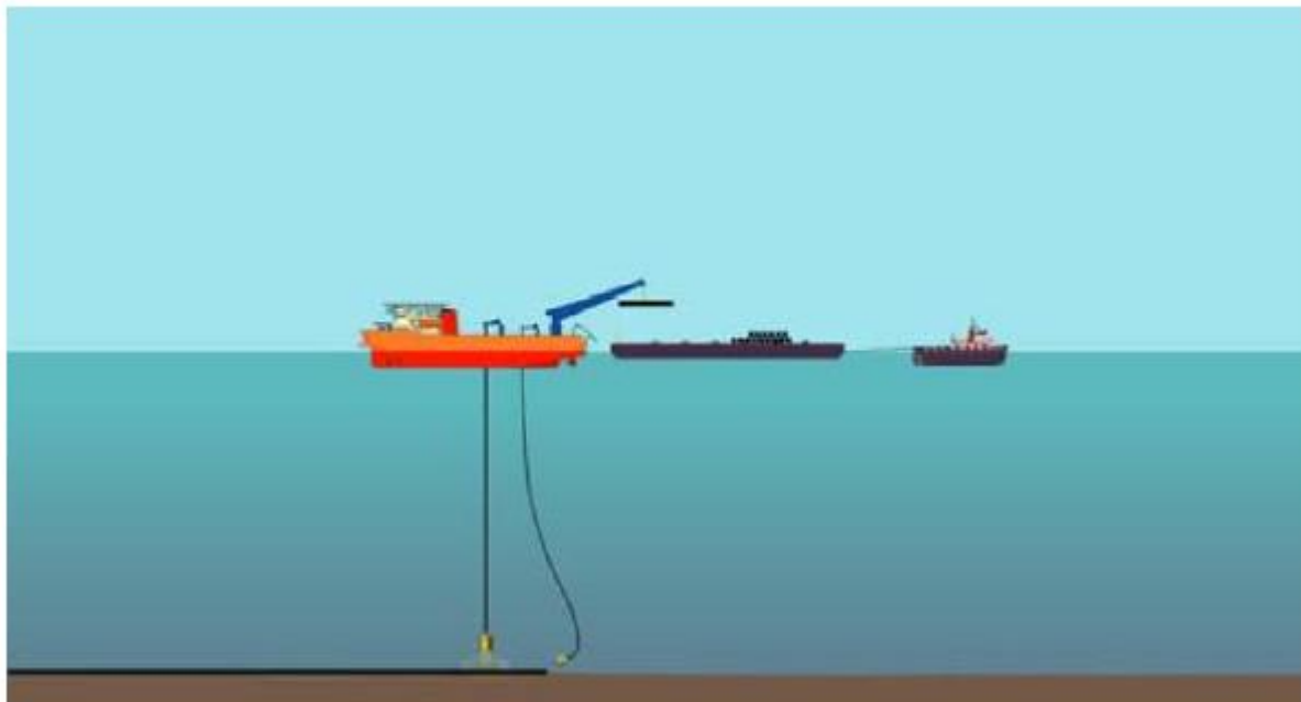
Figure 4-1 – Cut and Lift Pipeline Removal Illustration
