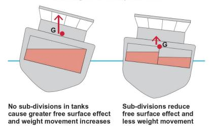
Longitudinal sub-divisions will reduce the free surface effect so the weight shift is drastically reduced.
