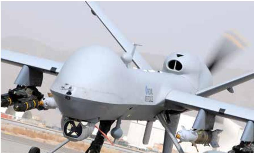
A Reaper MQ-9 remotely piloted air system prepares for take-off
