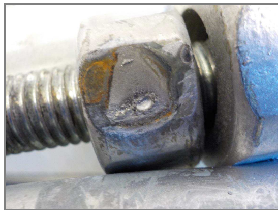
Fig.2 – close up of failed spot weld on nut showing reduced cross-sectional area of bonding
