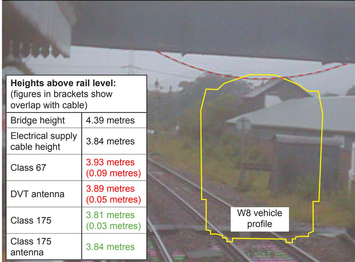
Figure 16: Vehicle heights above rail level in relation to the electrical supply cable drooping from the footbridge (background image courtesy of Arriva Trains Wales)
