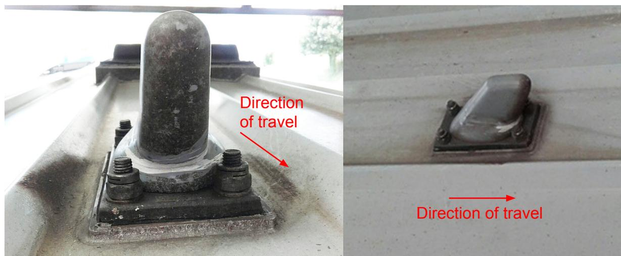
Figure 14: The radio antenna on the roof of the DVT (images courtesy of Arriva Trains Wales)
