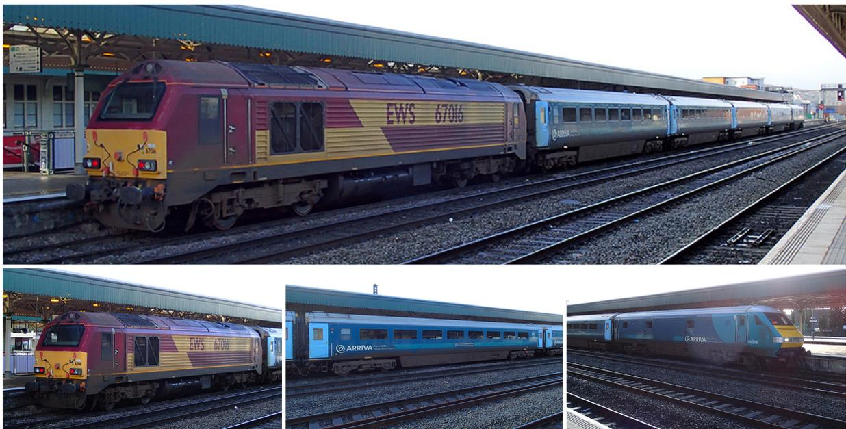
Figure 4: Class 67 locomotive, passenger coach and driving van trailer (DVT)
