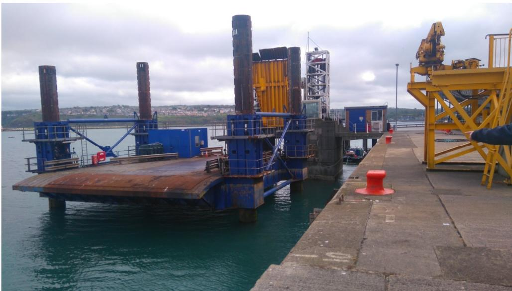
**Figure 2.7 Existing Jack Up Structure and piles**
