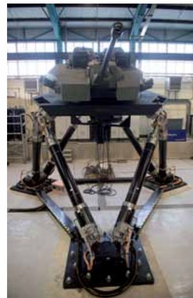
Above: latest addition to the programme is a £1 million motion test rig at Amptill to test turret stabilisation and performance. The rig will speed up development time, saving the costs of putting a real vehicle on a test track
