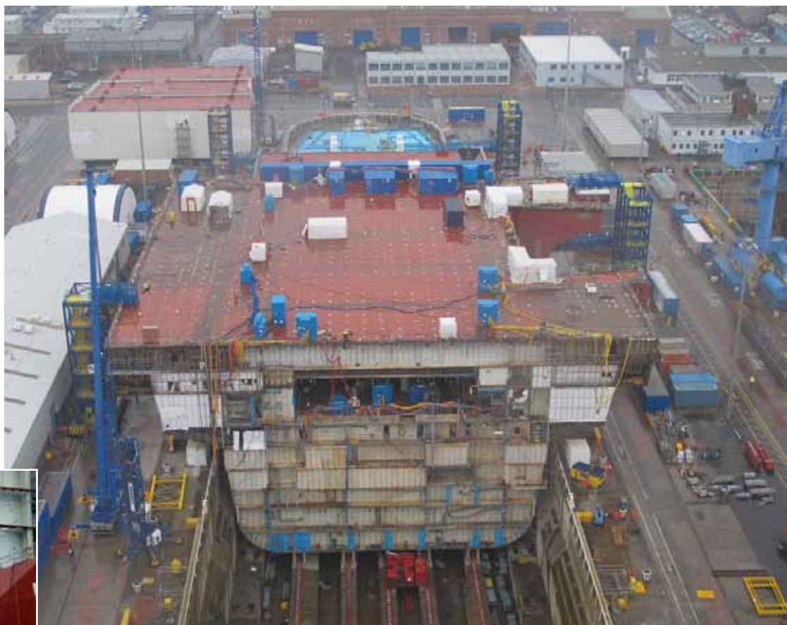
Progress: Queen Elizabeth takes shape at Babcock's yard in Rosyth as the second assembly cycle gets underway
