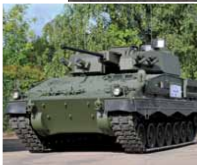
Flashpoint: Scout's armour system – modular armour packs bolted onto a hull – survives another test blast
