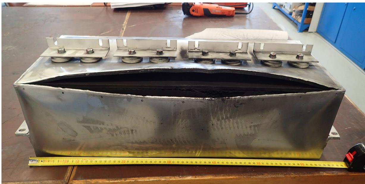
Figure 8: The damaged capacitor removed from coach 62826 prior to examination at Electronicon's facilities in Germany
