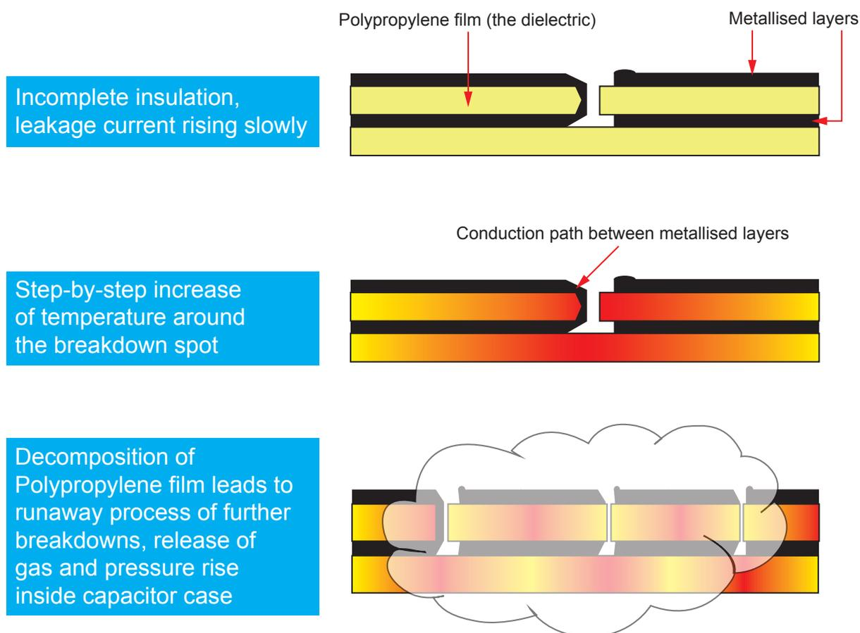
Figure 7: Drawing illustrating failure of self-healing
