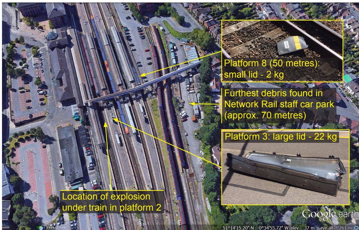
Figure 3: Locations of debris found after the explosion
