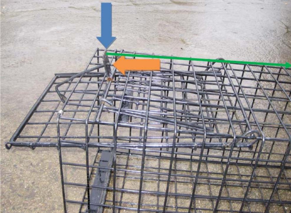
**Plate 1:** Trigger mechanism of trap showing hinge plate in roughly vertical position (blue arrow) and tip of trigger arm passed through lower hole of hinge plate (orange arrow) to hold trap door open. The green arrow indicates the line of twine, once set, from the upper hole of the hinge plate, running towards rear of trap.
