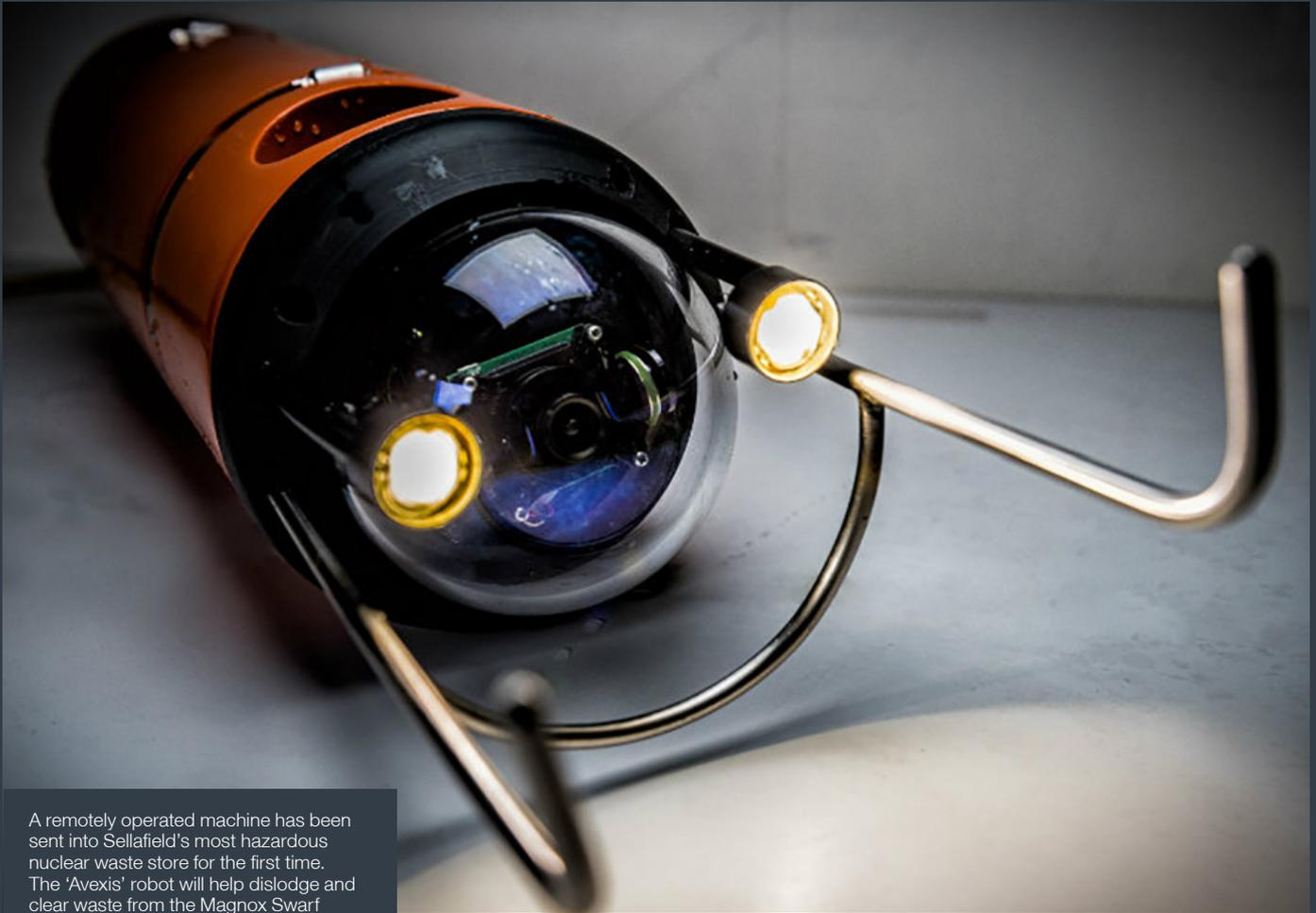
A remotely operated machine has been sent into Sellafield's most hazardous nuclear waste store for the first time. The 'Avexis' robot will help dislodge and clear waste from the Magnox Swarf Storage Silos.
