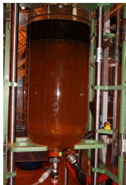
Rig used for high alpha oil treatment
