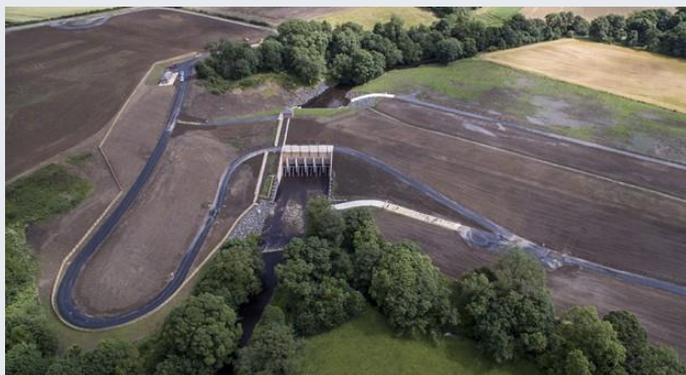
The scheme opened in August 2015, at a cost of £26m, (including £12m from Northumberland County Council). It includes one of the largest flood storage reservoirs the Environment Agency has ever built and reduces the risk of flooding to 1,000 homes and businesses in the area. The upstream dam and storage area on the Mitford Estate works by
