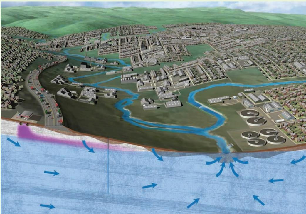
**Figure 4:** Illustration of conceptual model of fuel release to groundwater (copyright SNIFFER, 2005).
