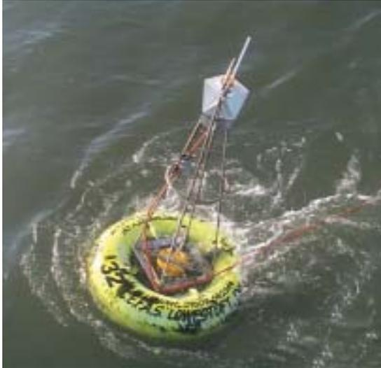
Smart buoy – providing real-time monitoring of the marine environment
