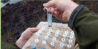
The gas is then transferred in to a vial. Samples are taken every 5 minutes over a 15 minute period for each sample site. These vials are later sent off to be analysed in a lab.
