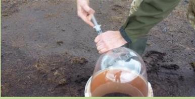
Air tight chambers are placed on the peat and gas samples are taken using a syringe. Samples are taken from transparent (see picture) and dark chambers, allowing us to compare the effects of photosynthesis on carbon uptake and release.
