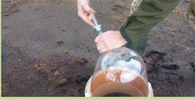
Air tight chambers are placed on the peat and gas samples are taken using a syringe. Samples are taken from transparent (see picture) and dark chambers, allowing us to compare the effects of photosynthesis on carbon uptake and release.
