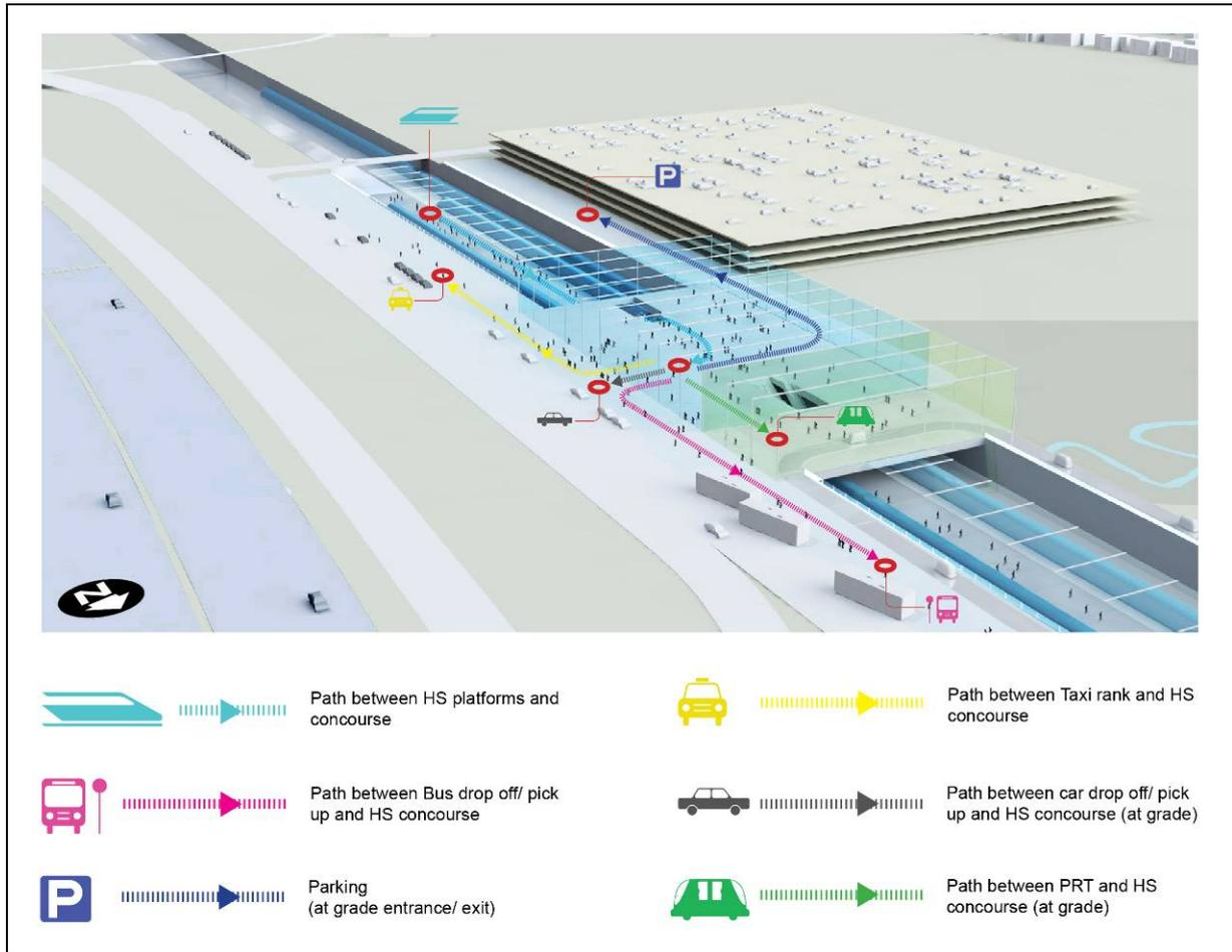
Figure 3.58: Interchange Option 4e - Intermodal Interchange Diagram
