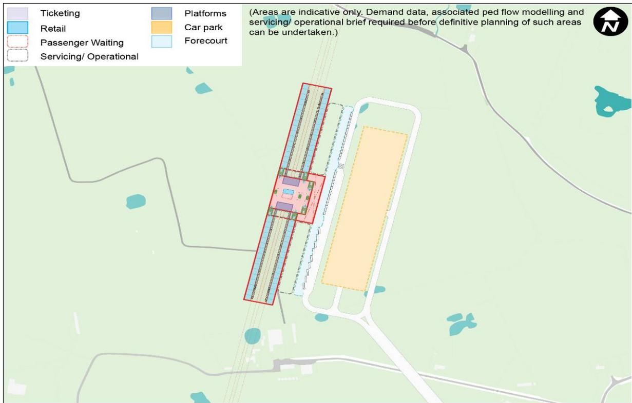
Figure 3.67: Interchange Option 5a - Concourse Level Plan
