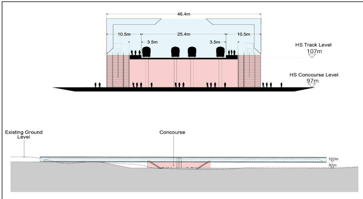
Figure 3.43: Intermediate Option - M6 – Cross And Long Sectional Views Of Proposed Station
