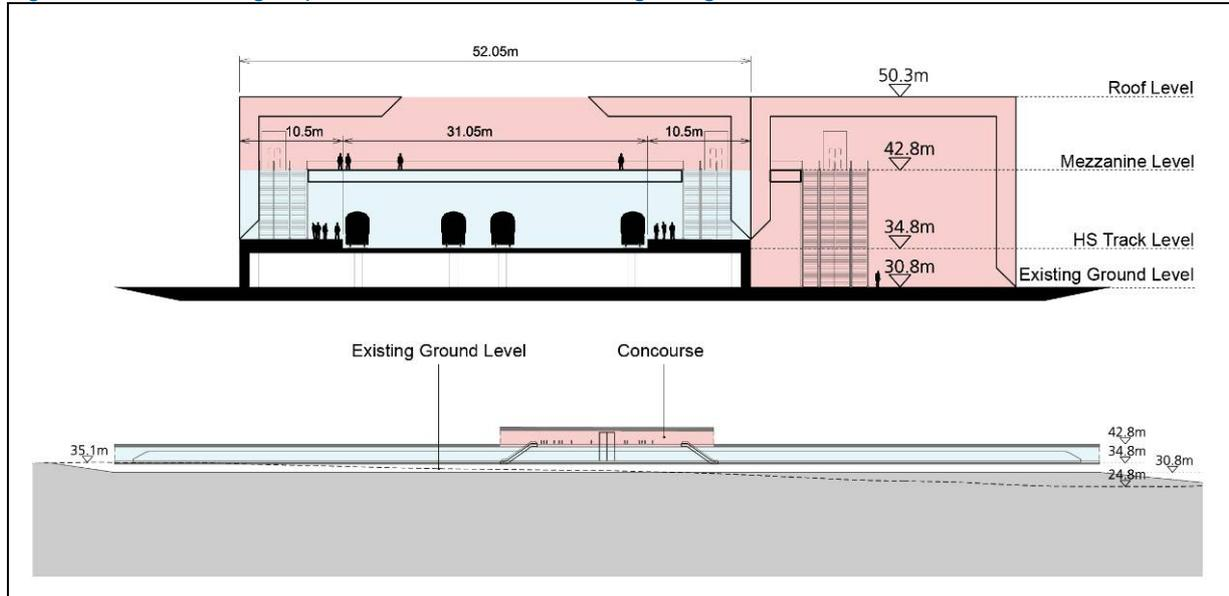
Figure 3.74: Interchange Option 30 - Sectional Views Of Proposed Station
