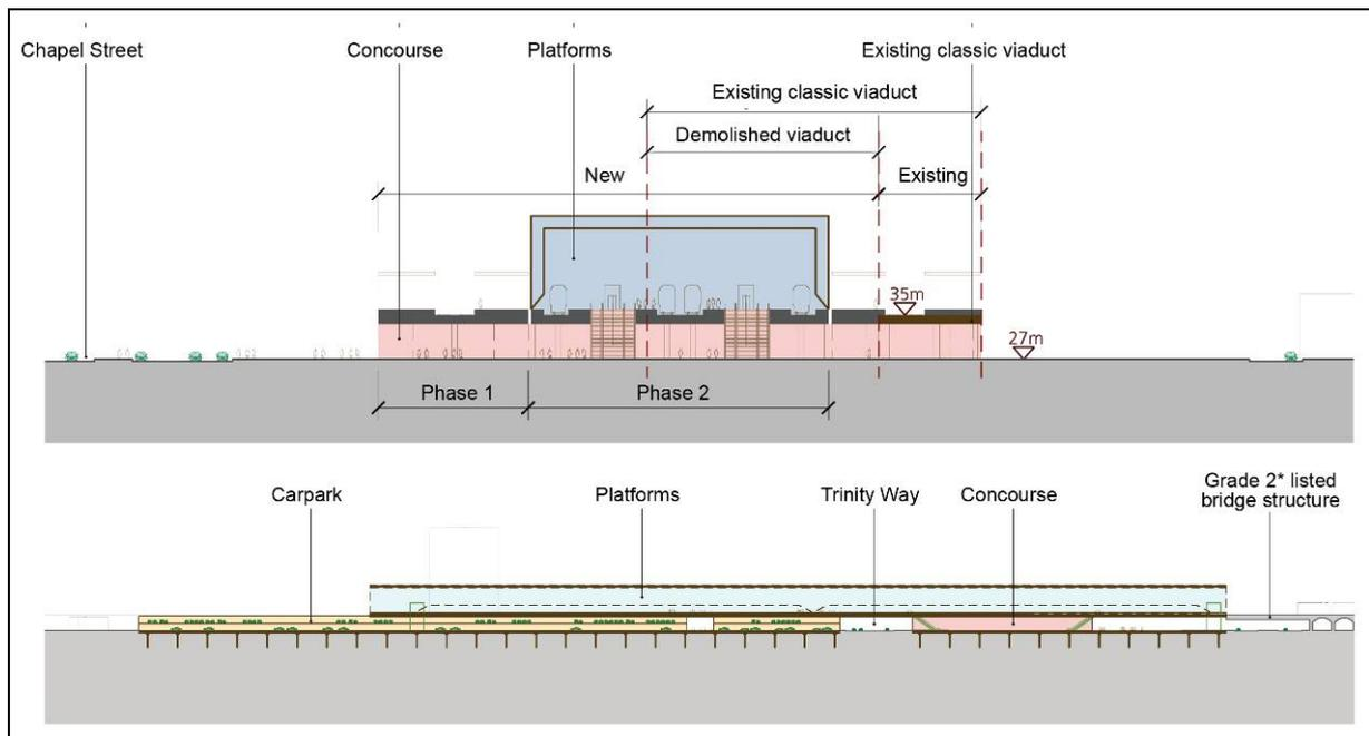
Figure 3.33: Option 19 – Cross And Long Sectional Views of Proposed Station
