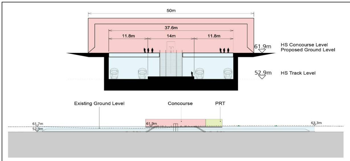
Figure 3.59: Interchange Option 4e - Sectional Views Of Proposed Station
