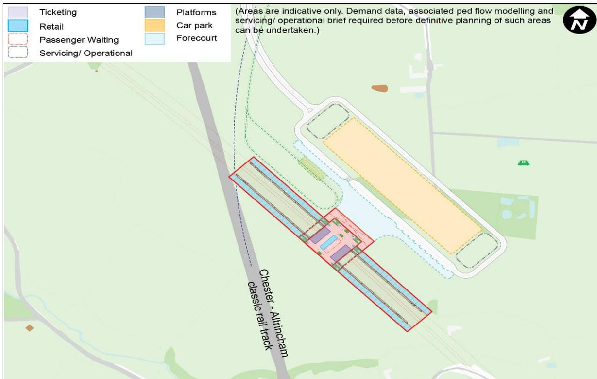
Figure 3.52: Interchange Option 4d- Concourse Level Plan
