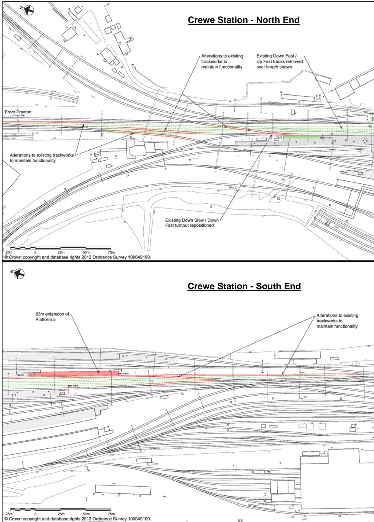
Figure 5.2: Crewe Station Reconfigured Track Layout
