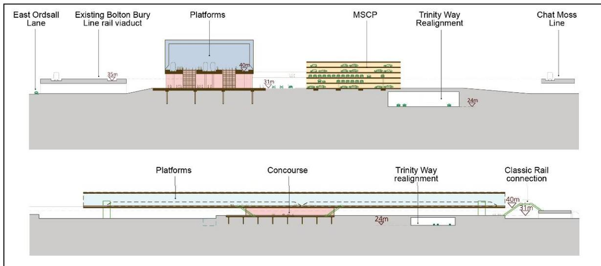
Figure 3.22: Option 9b – Cross And Long Sectional Views Of Proposed Station
