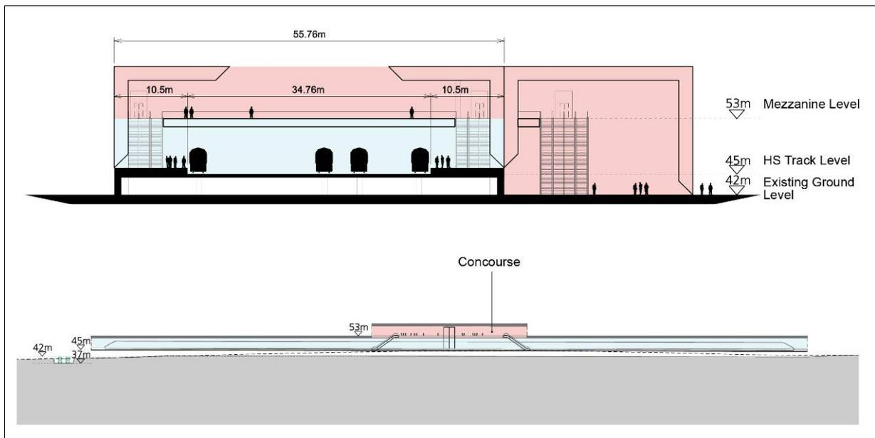
Figure 3.54: Interchange Option 4d – Cross And Long Sectional Views Of Proposed Station
