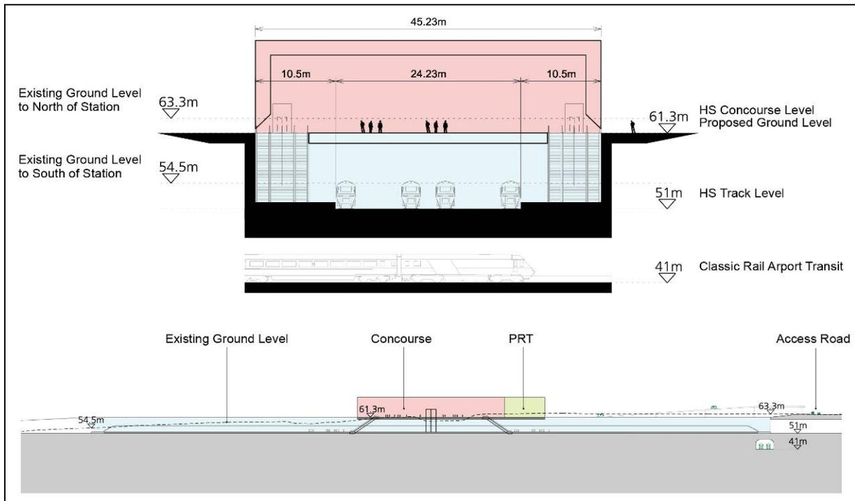
Figure 3.49: Interchange Option 4c – Cross And Long Sectional Views Of Proposed Station
