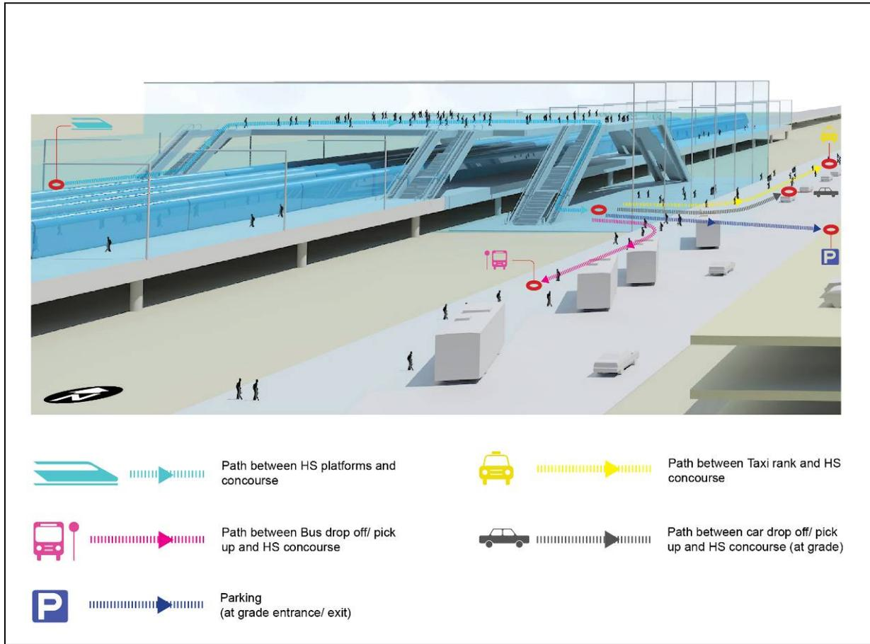
Figure 3.63: Interchange Option 5 - Intermodal Interchange Diagram
