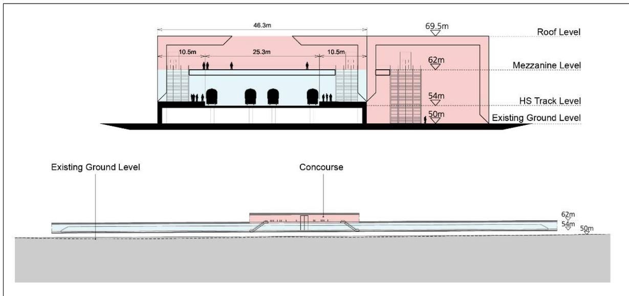
Figure 3.69: Interchange Option 5a - Sectional Views Of Proposed Station
