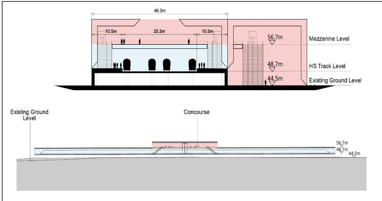
Figure 3.64: Interchange Option 5 – Cross And Long Sectional Views Of Proposed Station
