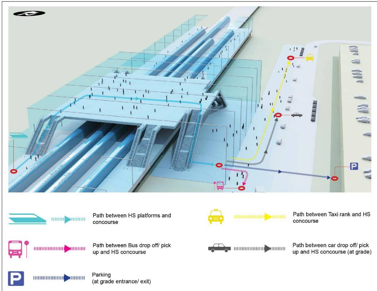
Figure 3.68: Interchange Option 5a - Intermodal Interchange Diagram
