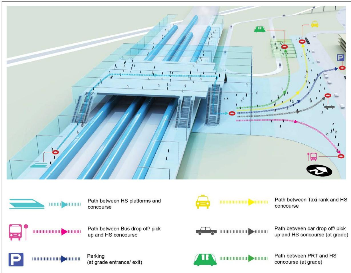
Figure 3.53: Interchange Option 4d - Intermodal Interchange Diagram
