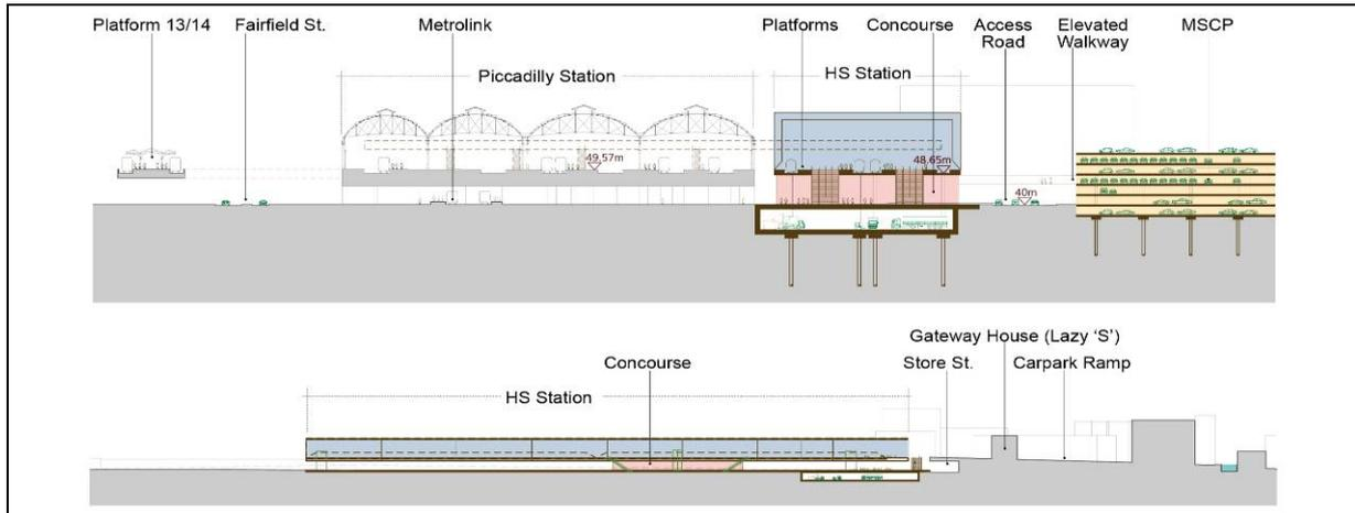
Figure 3.11: Option 1a – Cross And Long Sectional Views Of Proposed Station
