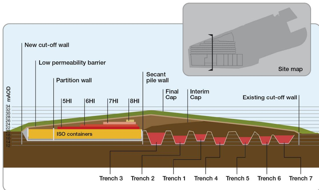
**Figure 4 Section across Vault 9 and the trenches**
