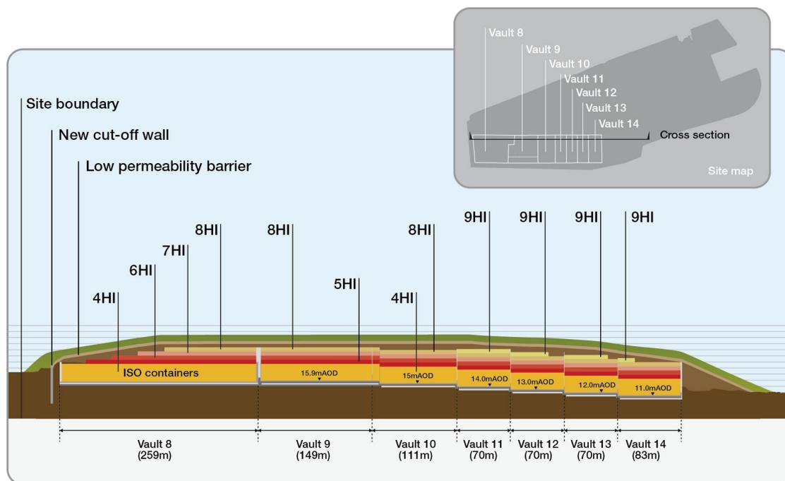
**Figure 5 Cross section along the vaults**
