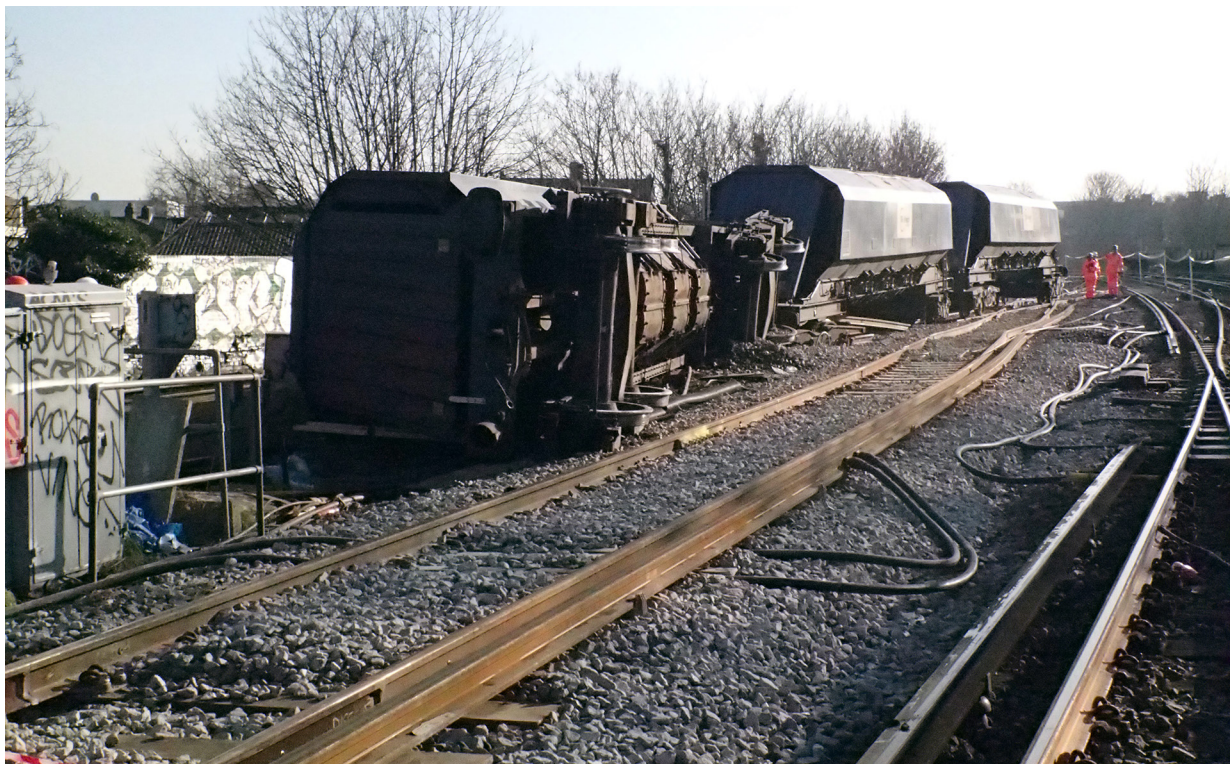
Figure 3: Location of the last three wagons of train 6M90 after the derailment
