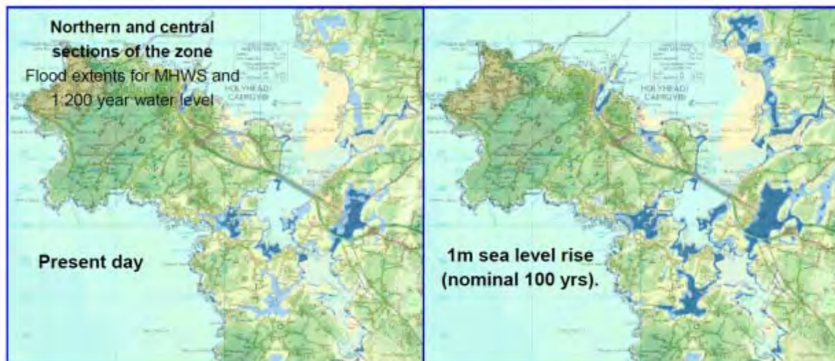
Figure 21-2 Predicted flood risk to Anglesey and Holyhead based on present data and on predicted 1m SLR (Source: Royal Haskoning, 2011a)
