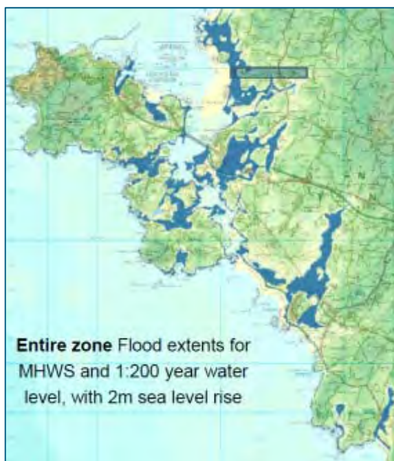
Figure 21-3 Predicted flood to Anglesey and Holyhead based on a predicted 2m SLR (Source: Royal Haskoning, 2011a)
