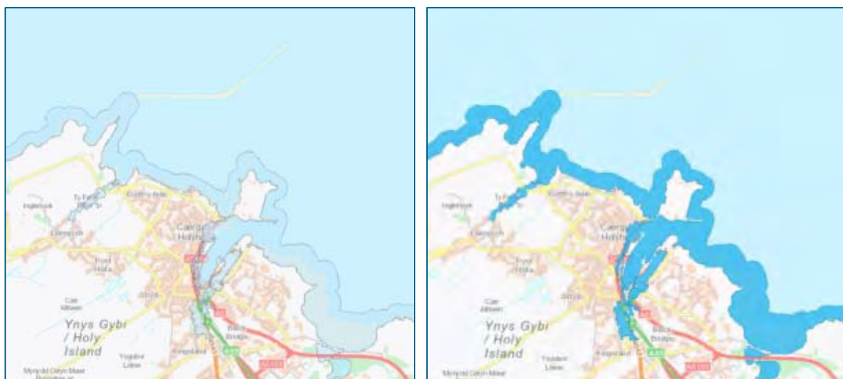
Figure 21-1 Extract from NRW flood risk map illustrating Flood Zone 2 (left image) and Flood Zone 3 (right image) (NRW, 2016b)
