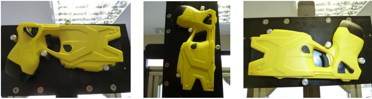
Figure B1: Shows the X2 in drop positions 1, 2 and 3 (left to right)
