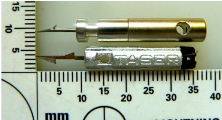
Figure 7: The standard X26 21ft operational probe (top) and the X2 25 ft SP barb probe (bottom)
