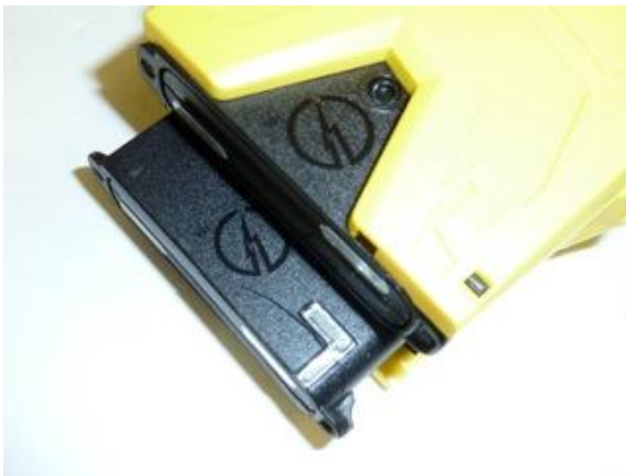
Figure B2: Damage to the X2 cartridge when dropped from position 2
