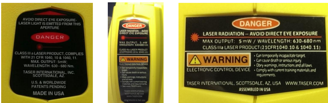
Figure 10: Examples of the label affixed to the X26, X26P and X2 (left to right)
