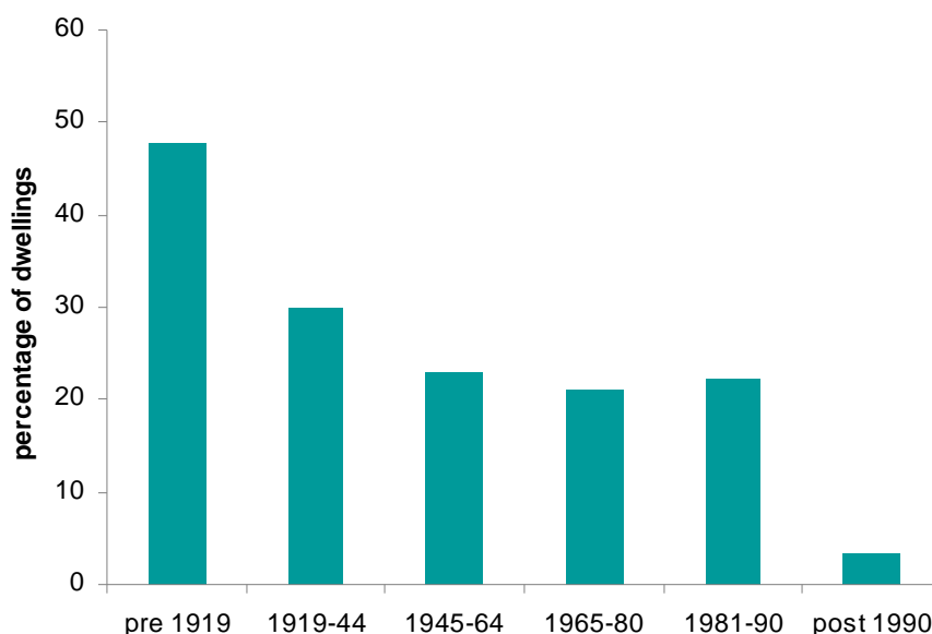
Figure 4.7: Dwellings failing Decent Homes by dwelling age, 2010
