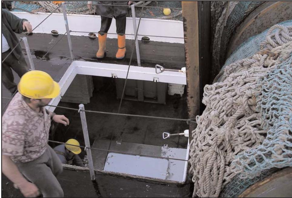
Using jury-rigged lifting gear on board a 35m trawler, two deckhands were being lifted out of the fish hold when they slipped and fell back down a distance of more than 4m. Both of the deckhands were taken to hospital with serious injuries.
