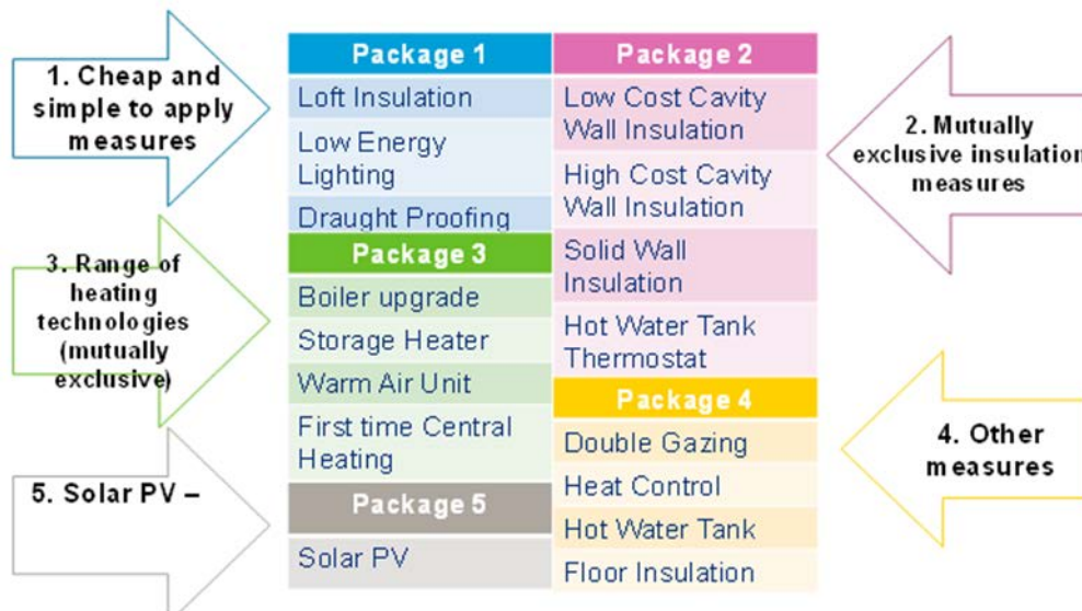
Figure C2a: Packages of measures that the NHM chooses from to install in PRS homes
