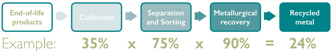
Figure 4: The recycling chain of end-of-life products. The total recycling efficiency of an end-of-life product is calculated by multiplying each of the single-stage efficiencies. This example shows indicative efficiency rates for the recovery of major metals (iron and steel, copper etc) found in waste electrical and electronic equipment (WEEE).
