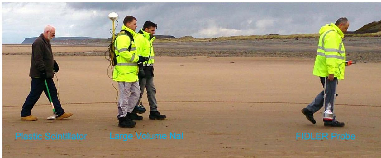
**Figure 27: Trials of a plastic scintillator detector on Sellafield Beach.**
