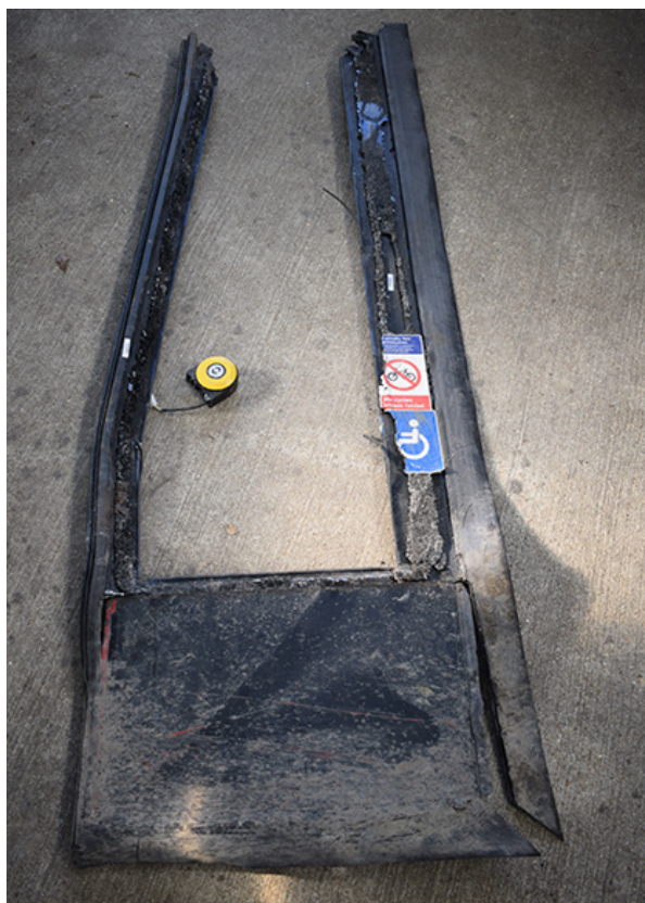
Figure 40: Typical door damage
