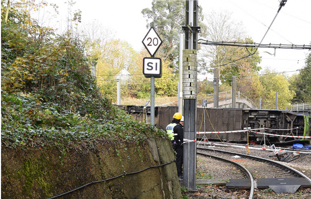
Figure 26: 20 km/h speed sign and 'SI' sign at the start of the west curve
