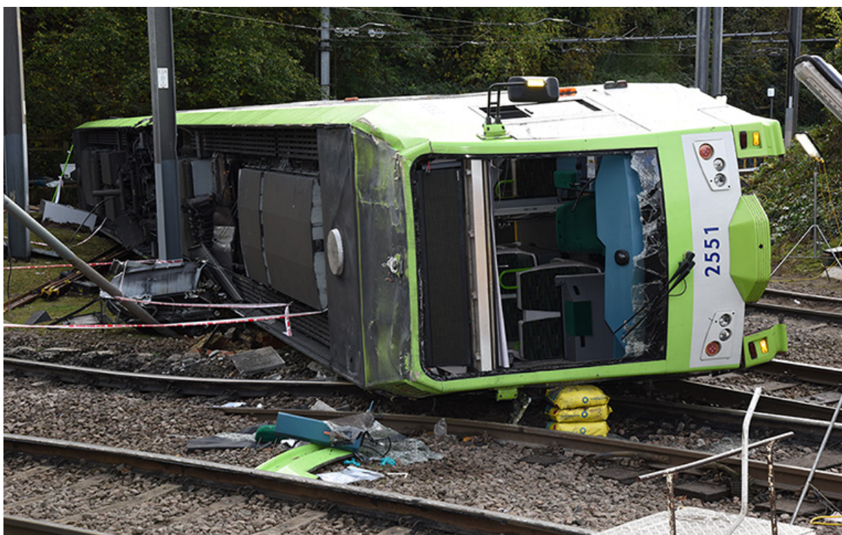
Figure 16: Front of tram with windscreen removed to evacuate passengers (initial hole formed by tram drivers/police officer, remainder removed by fire service)
