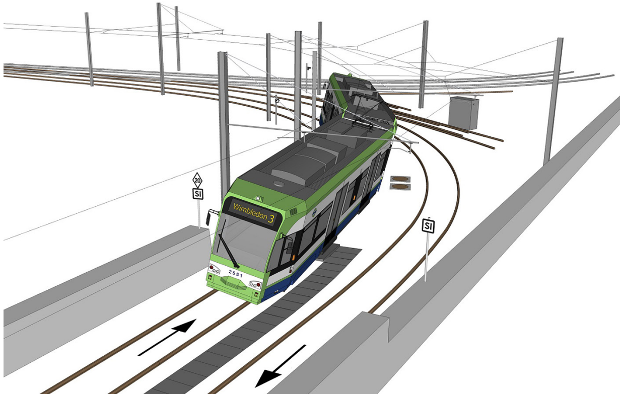
Figure G.1: Overview when front wheels become derailed (point of derailment). Tram is tilting over at about 10°. Note: the flexible connections between the sections of the tram are not shown for clarity.
