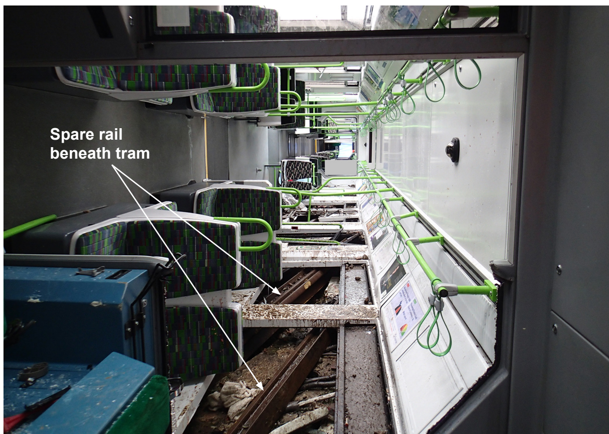
Figure 45: Tram 2551 overturned at accident site showing ground beneath broken windows (rails had been stored on the ground between the north and south curves before the accident, see figure 8)
