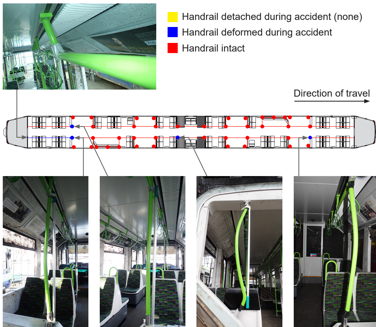
Figure 42: Extent of damage to handrails
