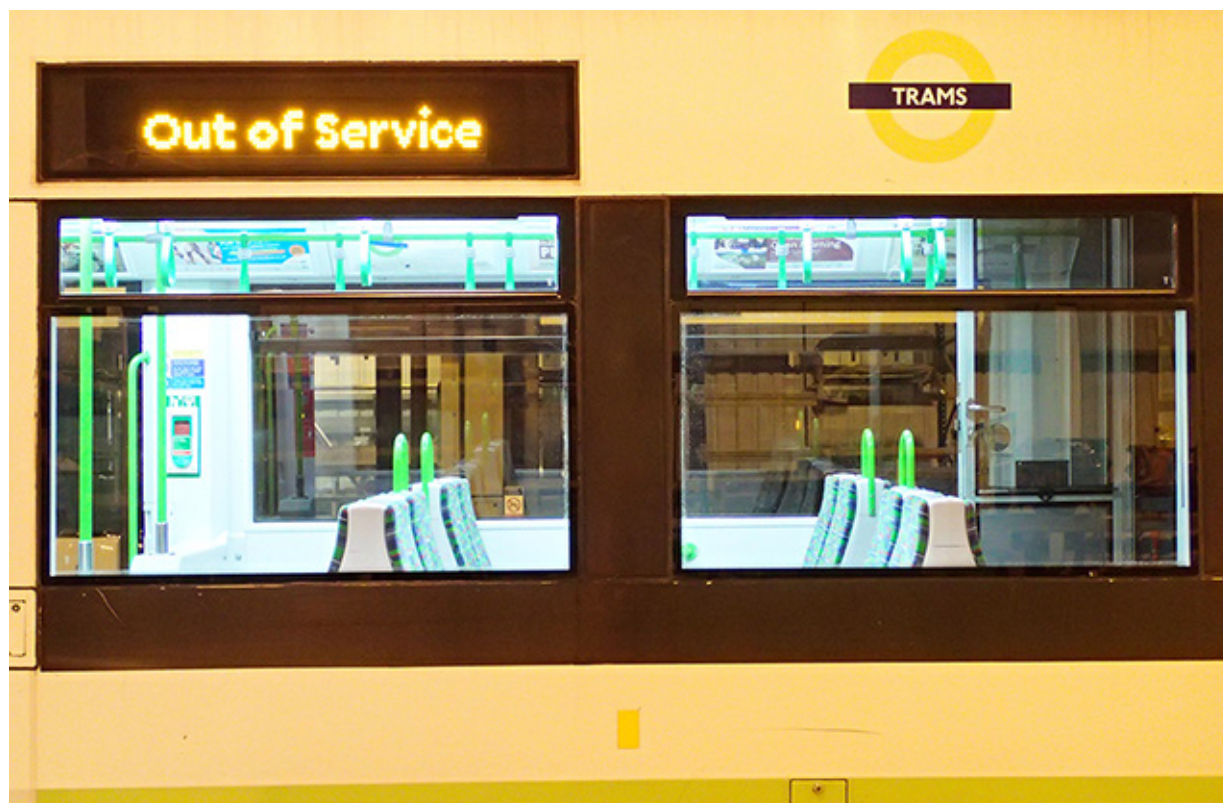
Figure 34: Typical window installation on a CR4000 tram
