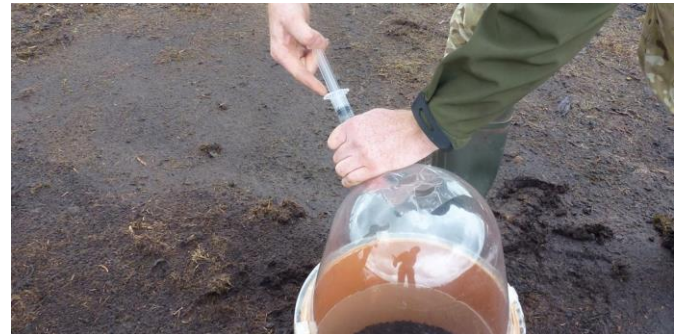
Gas samples are taken using a syringe. This photo shows one of the transparent chambers.
