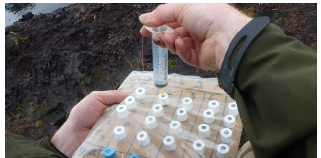
Gas is transferred into evacuated vials to send off for analysis.
