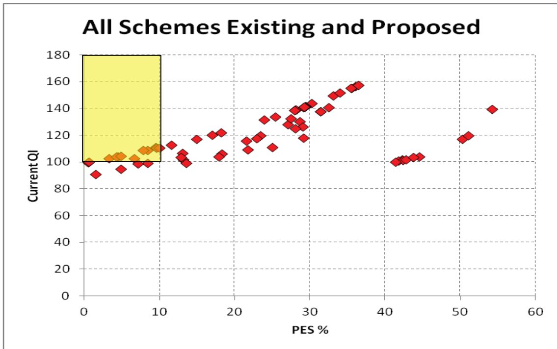
Figure 4. Current QI of all existing and proposed CHPQA certified schemes v Primary Energy Saving
