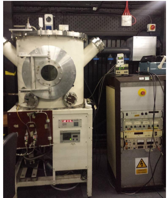
Figure 3.205 ECS spherical chamber for HC testing and vertical chamber for PPTs and HCTs
