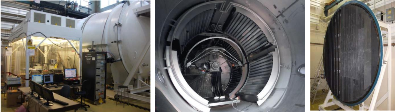
Figure 3.98 LEEP3 chamber showing T6 thruster installed and chevron target on door
