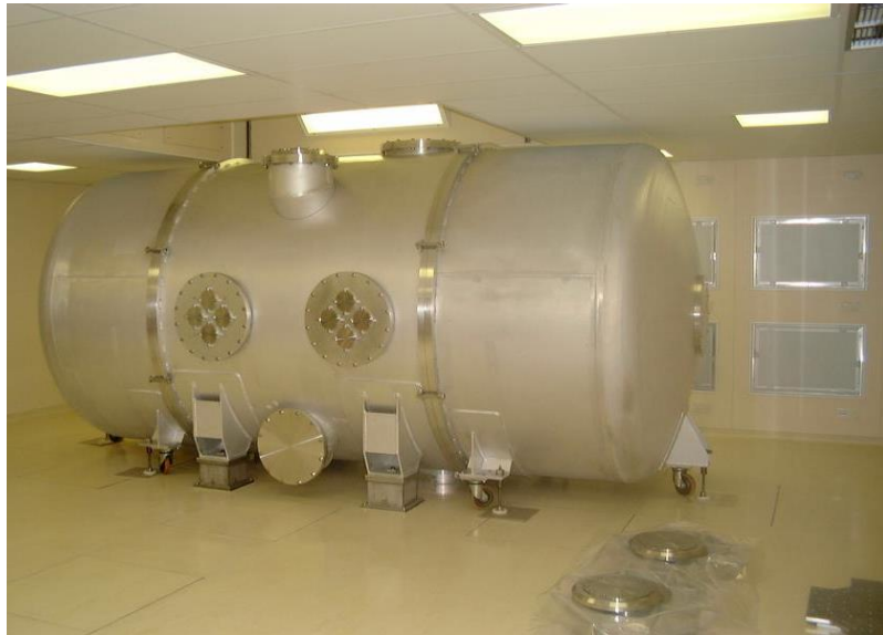
Figure 3.196 Oxford's 2.2m low-vibration TVAC chamber
