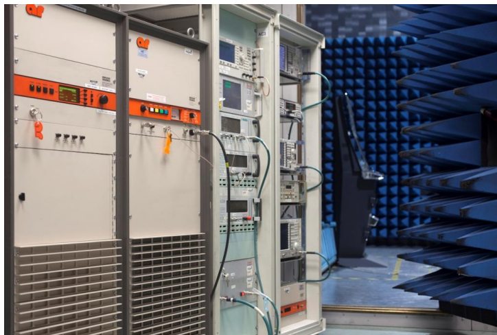
Figure 3.21 Typical 3C Test Anechoic Chamber
