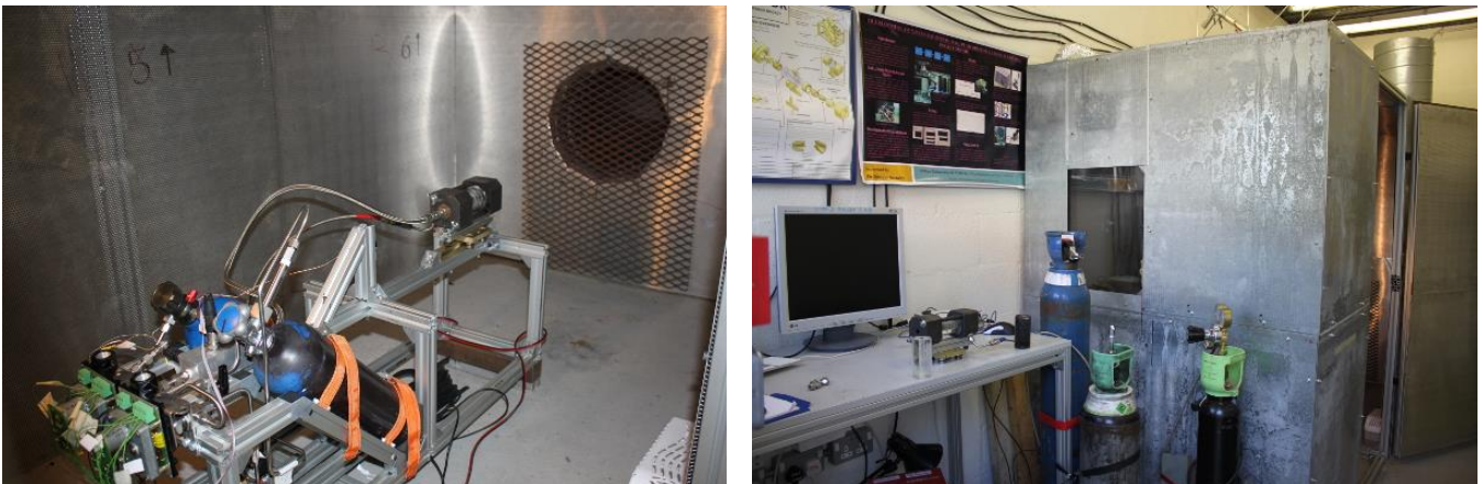
Figure 3.187 Bi-propellant rocket engine in Kingston's rocket test cell and external view of cell
