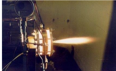
Figure 3.212 Surrey hybrid rocket engine firing
