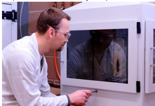
Figure 3.175 Single Burning Item Test and Single flame source
