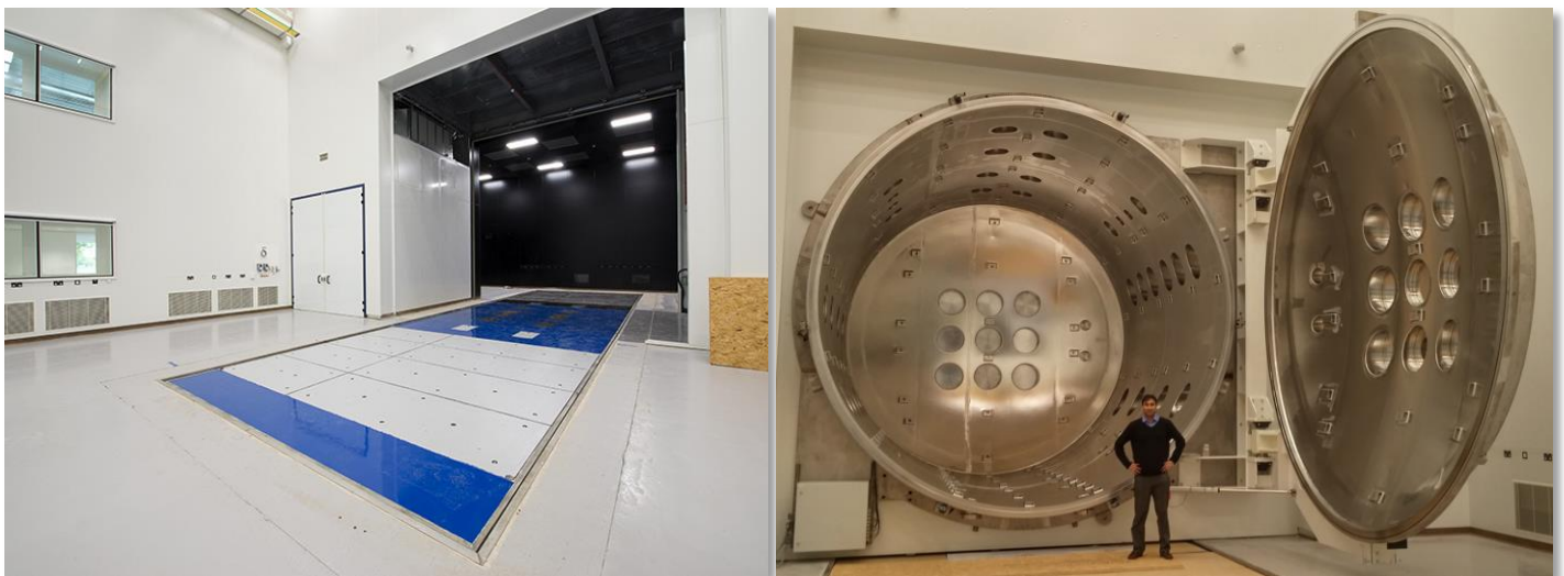
Figure 3.114 Clean room suite and seismic block prior to installation and 5m TVAC chamber newly installed
