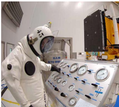
Figure 3.17 ADS-S Propulsion System Test and Propellant Loading
