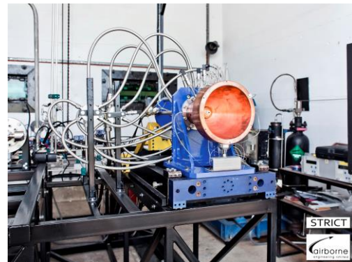
Figure 3.3 Lapcat engine firing and STRICT expansion-deflection research nozzle in AEL's J2 Test Bay
