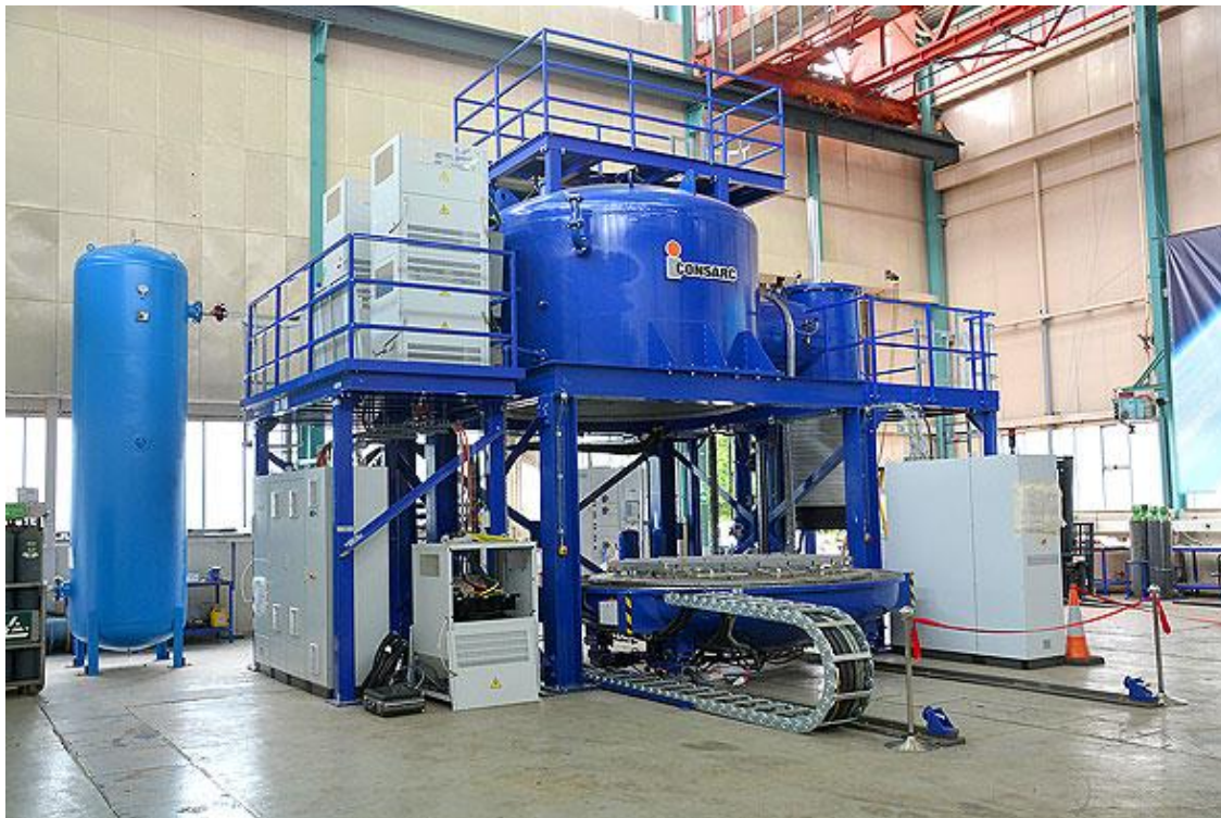
Figure 3.129 REL’s new vacuum furnace
