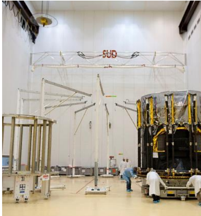
Figure 3.92 GAIA sunshield deployment gravity compensation facility
