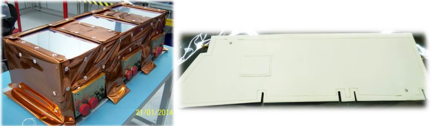
Figure 3.125 EarthCARE battery MLI (left) and EarthCARE BBR Beta cloth MLI (right)
