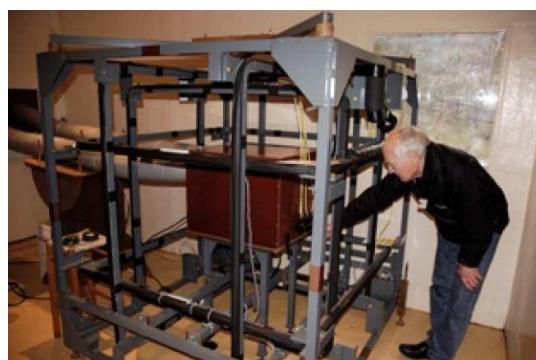
Figure 3.64 Imperial's 3-axis Helmholtz coil magnetometer calibration facility in Staffordshire
