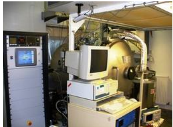
Figure 3.181 MSSL TVAC chamber
