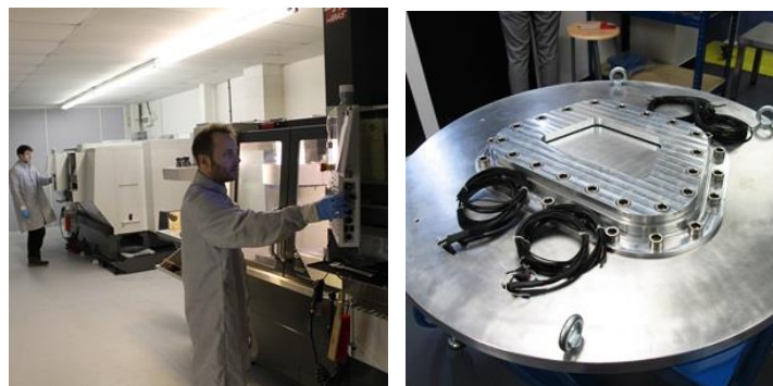
Figure 3.72: Rapid prototyping facility and destructive testing of window for manned spaceflight
