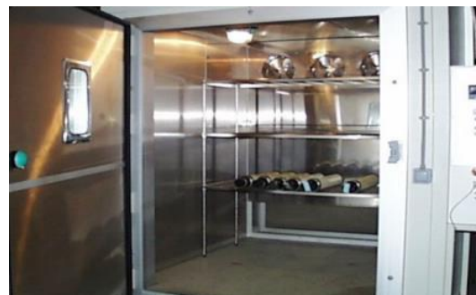
Figure 3.144 Typical environmental chamber
