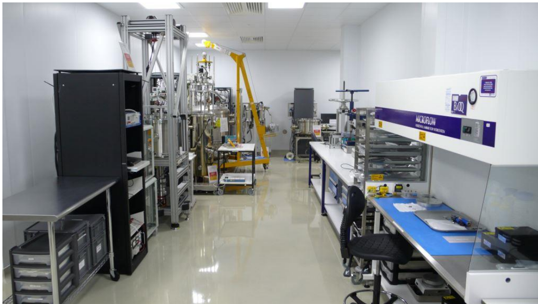
Figure 3.48 ESR Cleanroom mechanism assembly area and Class 100 bench
