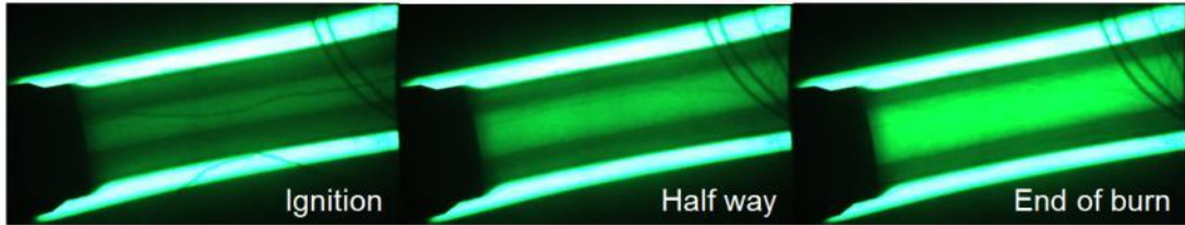
Figure 3.141 Insulation erosion during firing from Real-Time X-ray (RTX)
