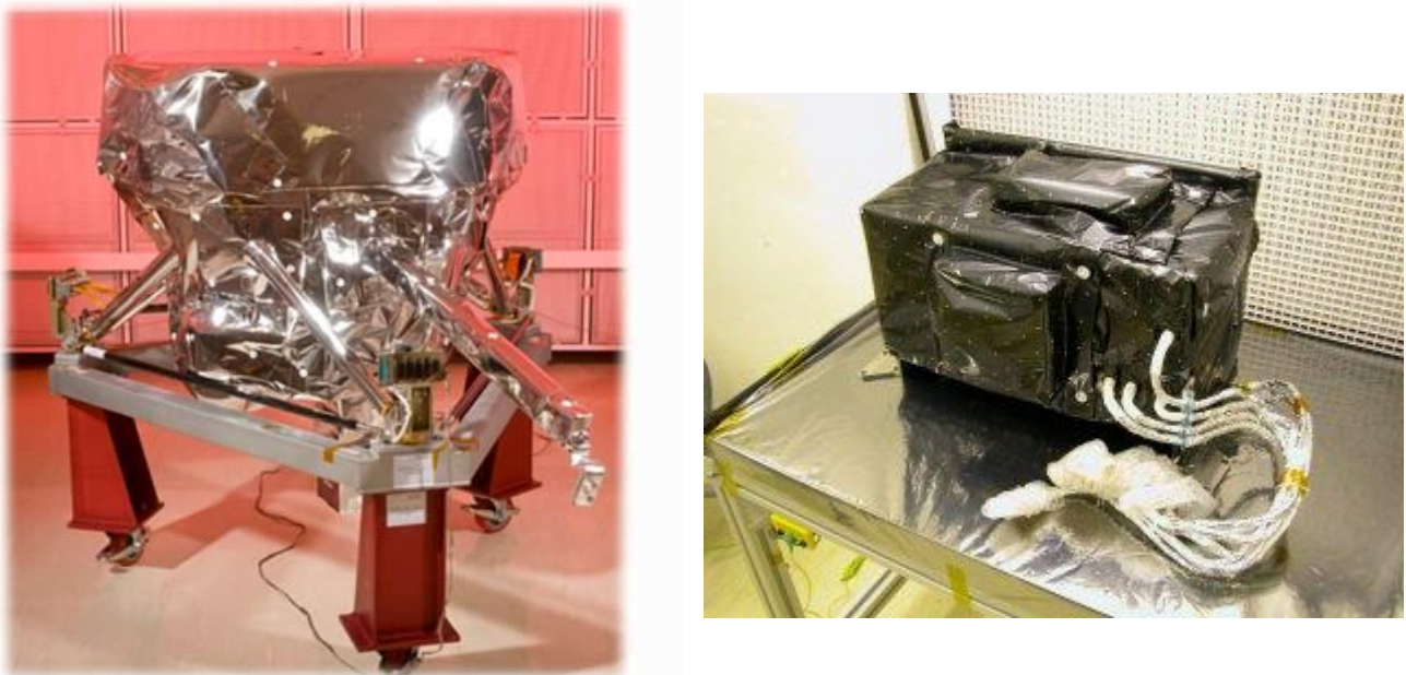
Figure 3.126 MIRI Cryogenic MLI (left) and GERB with MLI installed (right)
