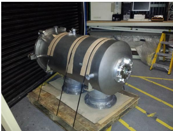
Figure 3.206 ECS large chamber for high power cathode development
