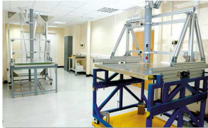
Figure 3.5 ADS-P Shock Test Facilities
