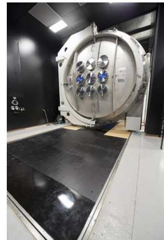
Figure 3.112 R100 clean integration areas at either end of the 5m chambers (during installation)
