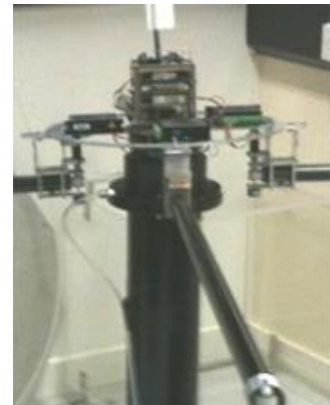
Figure 3.210 Air-bearing NanoSat Simulator
