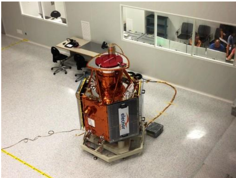
Figure 3.46 Deimos-2 FM spacecraft during final integration in Spain and in flight configuration
