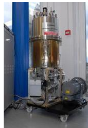
Figure 3.184 MSSL vacuum bakeout chamber
