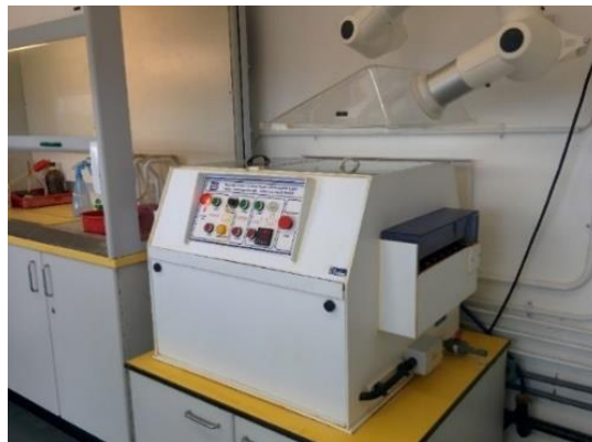
Figure 3.108 LITTLEJOHN UV exposure unit (left) and copper PCB etcher (right)
