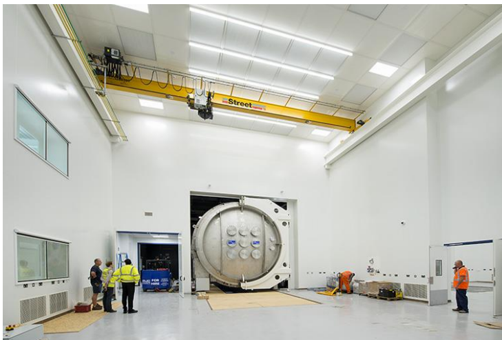
Figure 3.112 R100 clean integration areas at either end of the 5m chambers (during installation)
