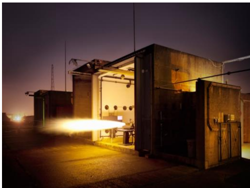
Figure 3.3 Lapcat engine firing and STRICT expansion-deflection research nozzle in AEL's J2 Test Bay
