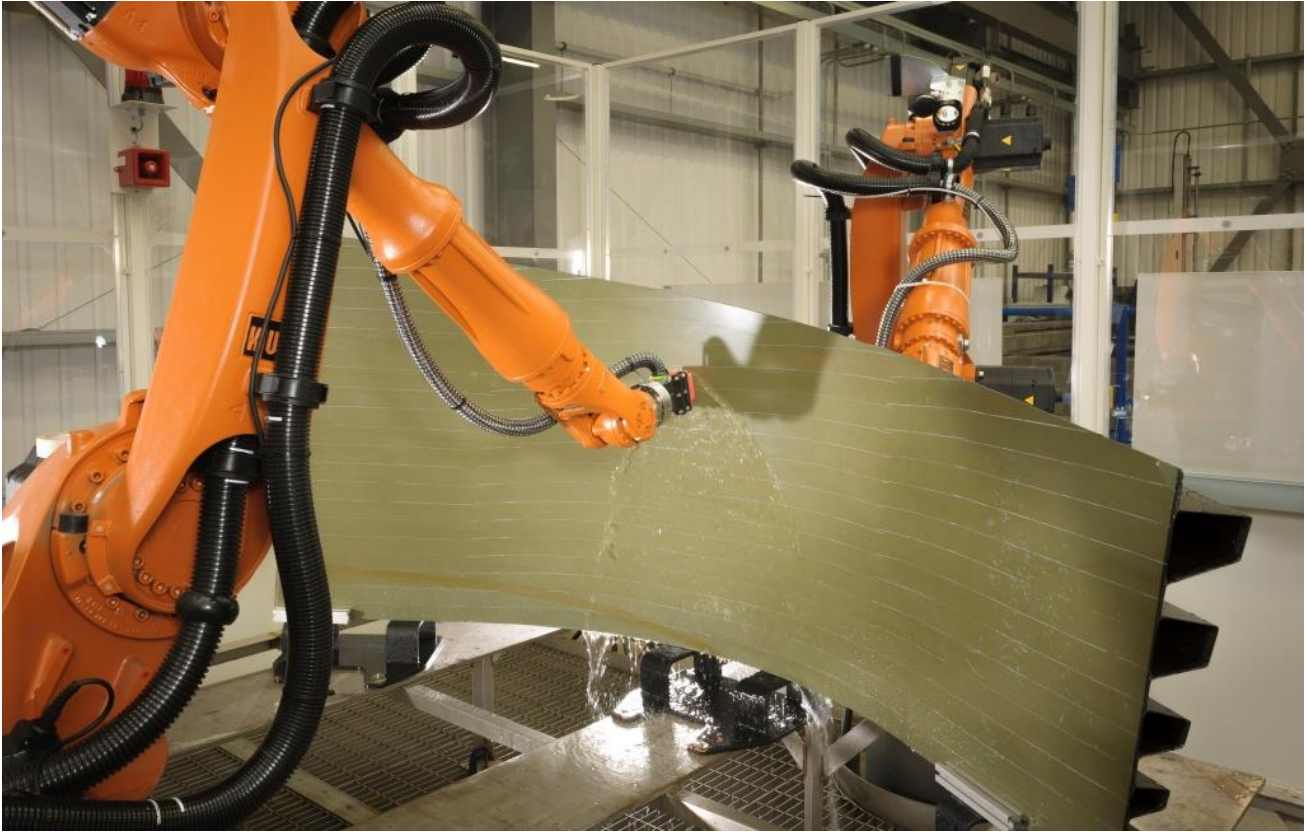
Figure 3.165 Robotic inspection of an aerospace component
