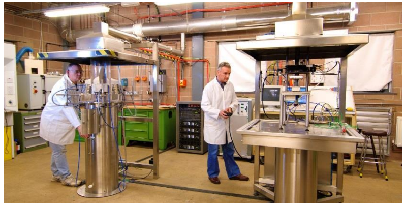
Figure 3.173 Resin transfer moulding system
