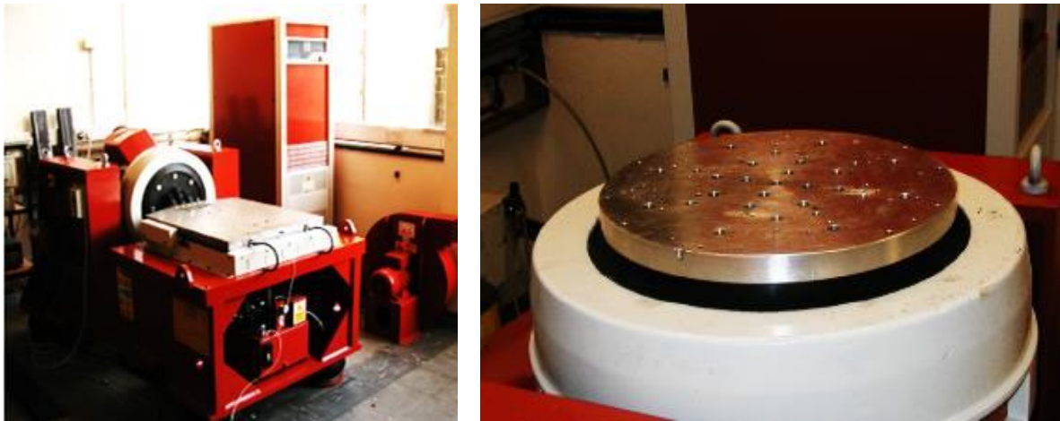
Figure 3.203 Vibration shaker in horizontal (left) and vertical configuration (right)
