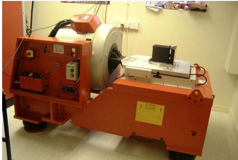
Figure 3.194 Oxford's 16kN LDS vibration facility
