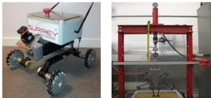
Figure 3.213: Examples of STAR Lab rovers and wheel soil interaction test rigs
