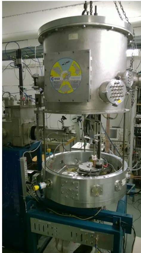
Figure 3.34 Heavy ion SE testing chamber used by Cobham at University of Jyväskylä
