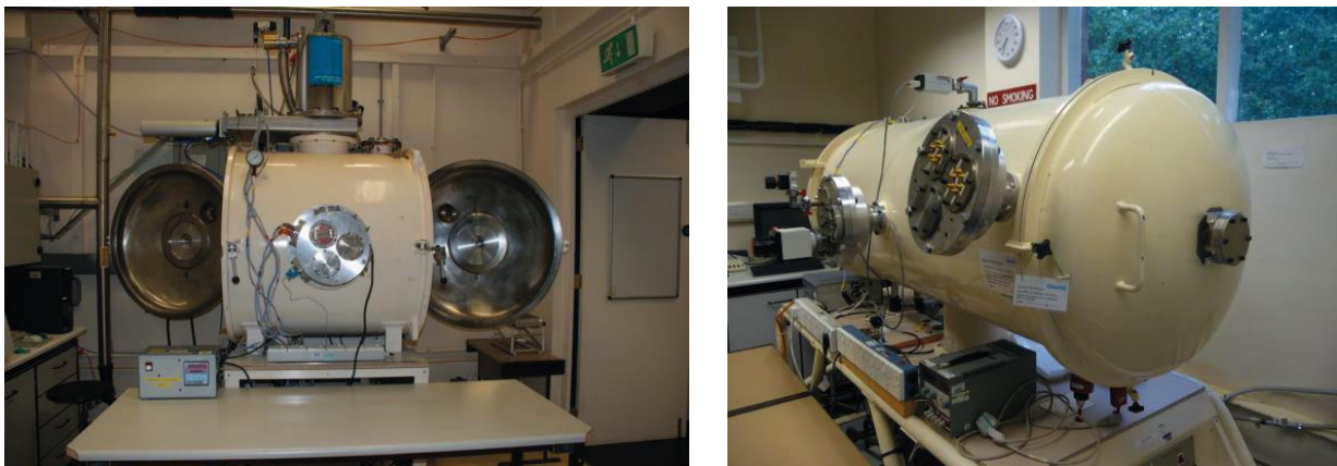
Figure 3.99 QinetiQ's 1m (left) and 0.5m (right) small EP TVAC chambers
