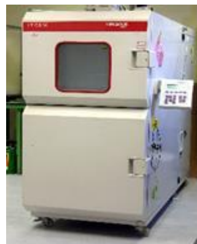
Figure 3.42 Edinburgh thermal shock chamber
