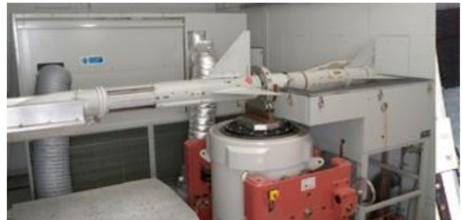
Figure 3.143 Rocket mounted on large vibrator
