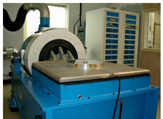
Figure 3.39 Aylesbury Vibration Test Facility
