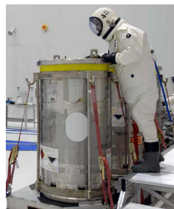
Figure 3.17 ADS-S Propulsion System Test and Propellant Loading
