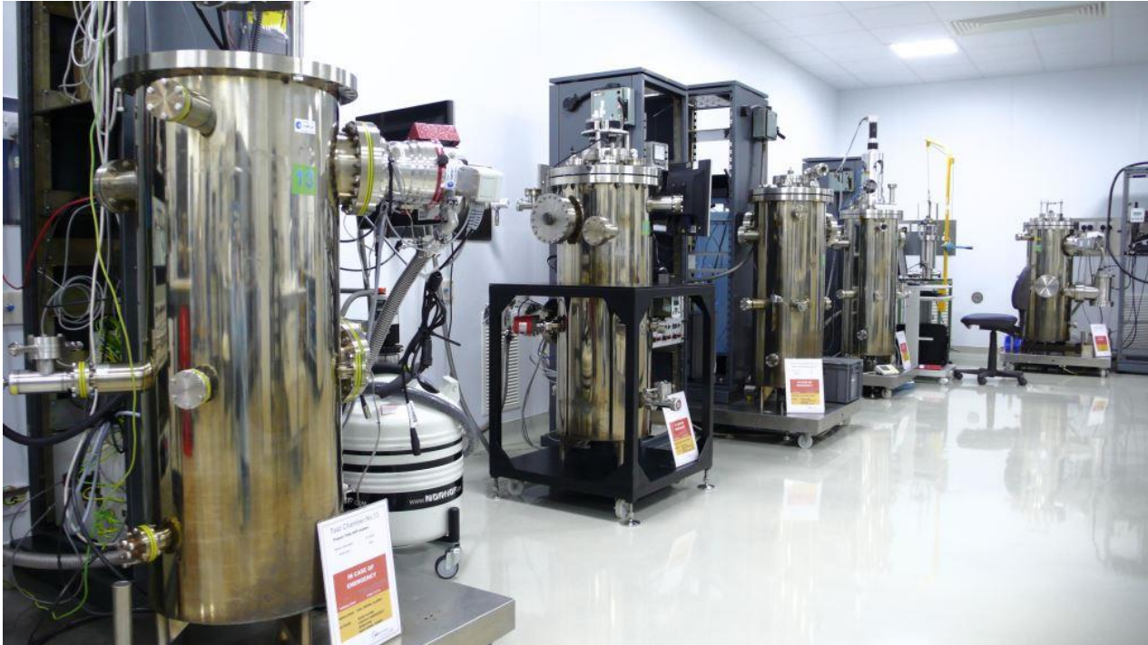
Figure 3.49 ESR thermal vacuum chambers
