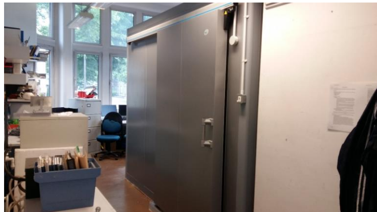
Figure 3.27 AIG large thermal test chamber
