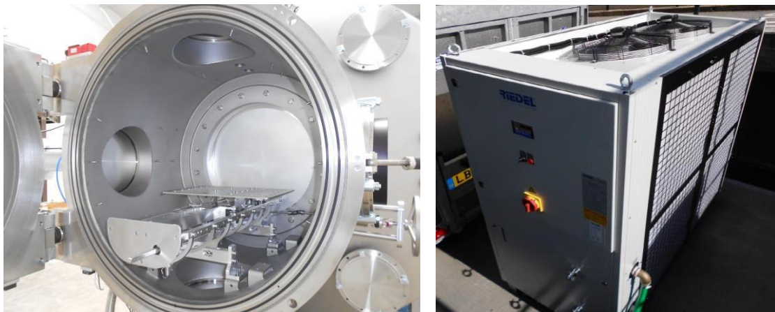
Figure 3.201 Loading chamber with traversing carriage (left) and high power chiller (right)
