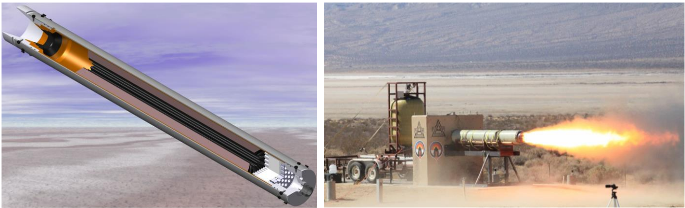
Figure 3.54 Cut-away of Falcon's hybrid rocket and test firing in the Mojave Desert
