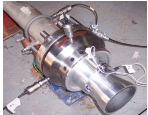
Figure 3.145 Cold gas thruster testing air rig
