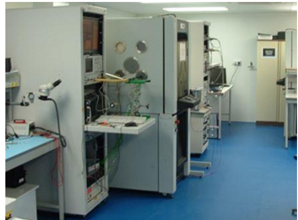
Figure 3.40 Aylesbury thermal test chambers
