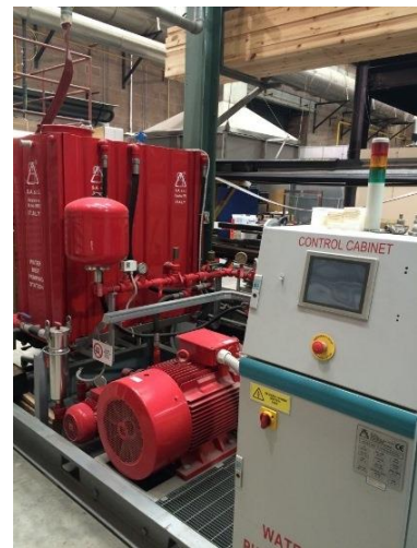
Figure 3.174 FireSERT's 20MW 9m x 9m large burn hood and 100 bar water mist system
