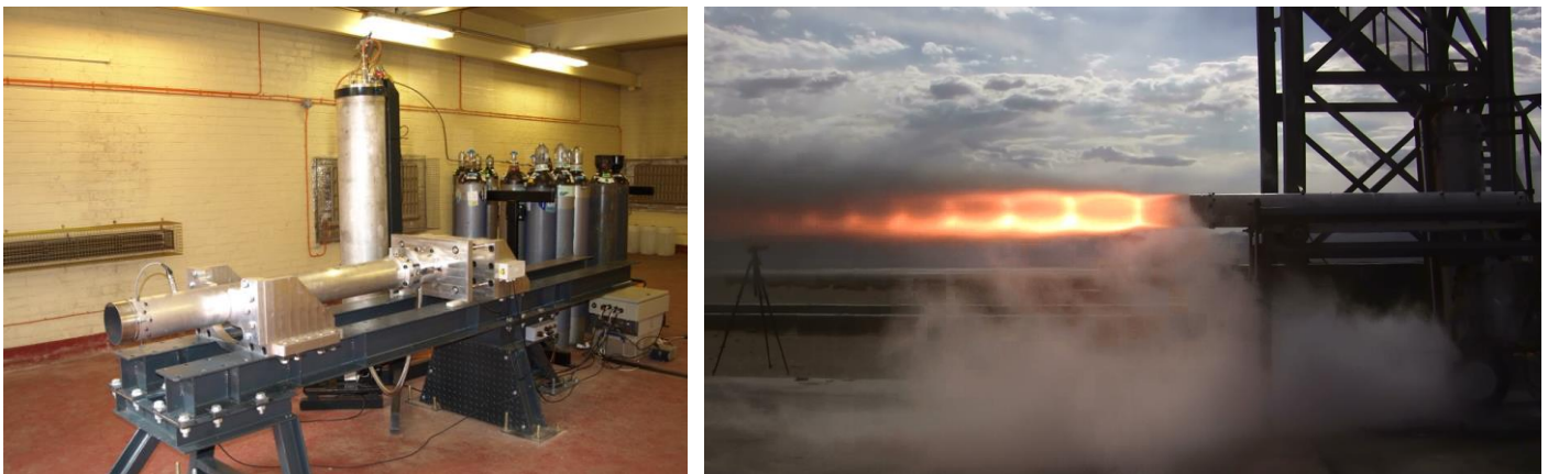
Figure 3.55 6-inch hybrid rocket on test-stand at Westcott and 6-inch rocket motor test firing
