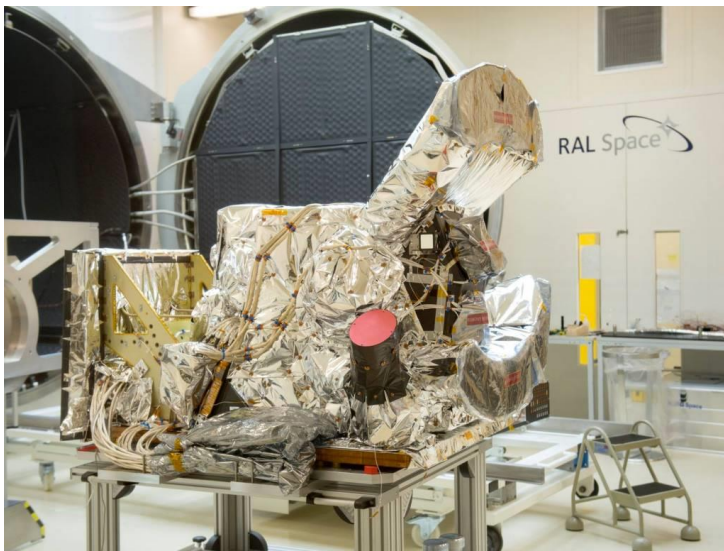
Figure 3.117 SLSTR calibration in RAL Space 3m Space Test Chamber
