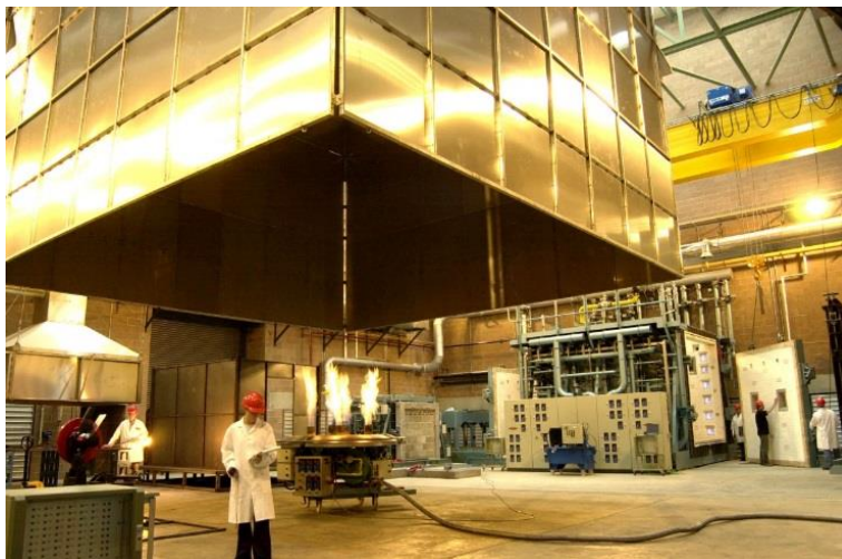
Figure 3.174 FireSERT's 20MW 9m x 9m large burn hood and 100 bar water mist system
