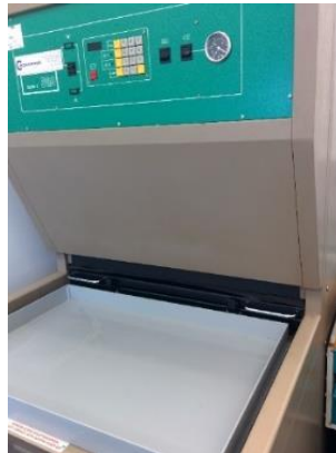
Figure 3.108 LITTLEJOHN UV exposure unit (left) and copper PCB etcher (right)
