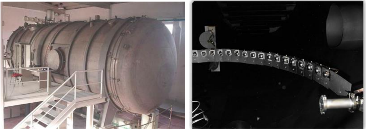
Figure 3.94 Aerospazio’s LVTF-1 EP chamber and boom-mounted Faraday probes in Siena
