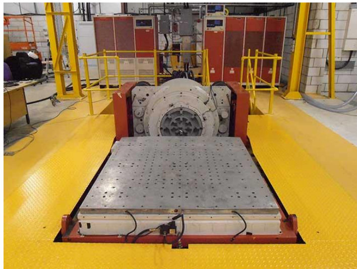
Figure 3.47 Element LDS V984 Electromagnetic Shaker
