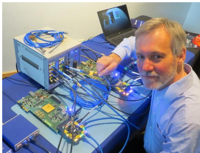
Figure 3.156 Demonstrating SpaceFibre, the next generation of SpaceWire technology
