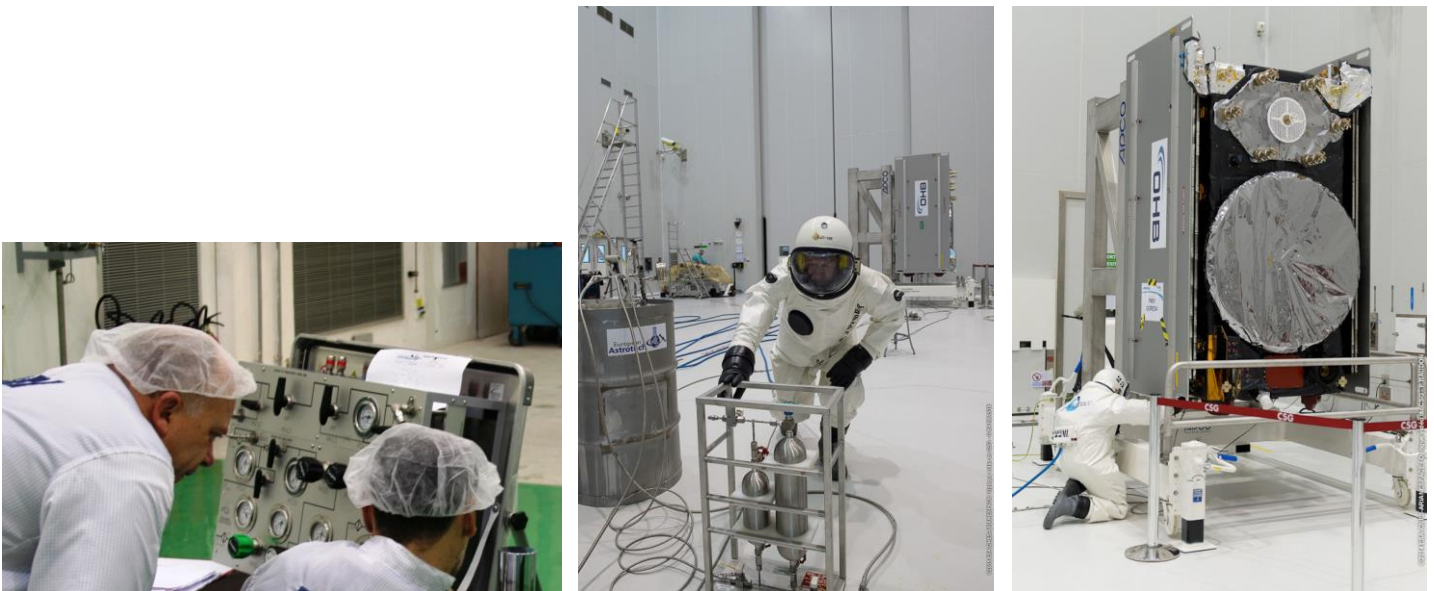
Figure 3.53 EAL propellant-loading GSE and loading the Galileo spacecraft at CSG
