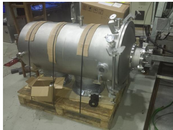
Figure 3.206 ECS large chamber for high power cathode development
