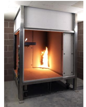
Figure 3.174 FireSERT's 20MW 9m x 9m large burn hood and 100 bar water mist system
