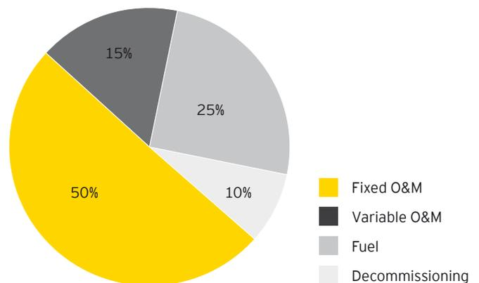
Figure 19 - Breakdown of operating expenditure for large reactors<sup>4</sup>
