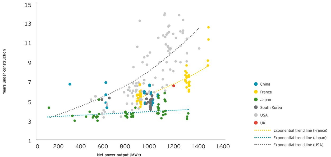
Figure 11 - Effects of size and approach on large reactor (PWR) construction schedules<sup>20</sup>
