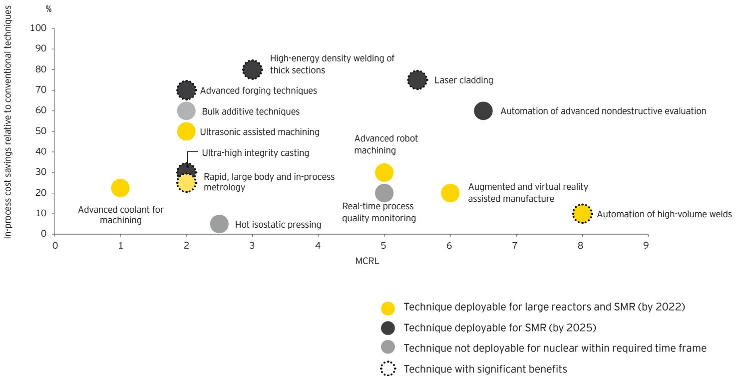
Figure 15 - The in-process savings for each technique against the maturity of the process
