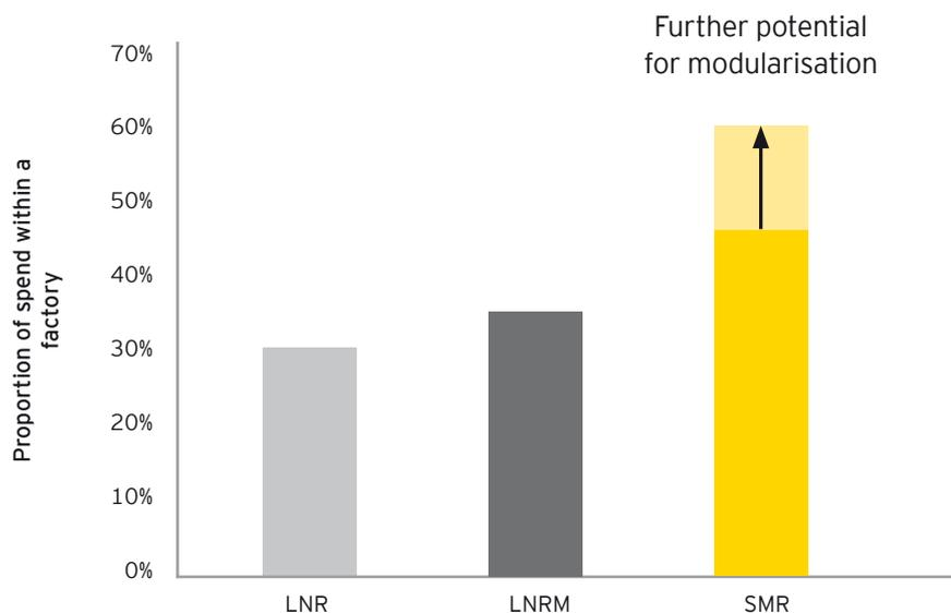
Figure 6 - Proportion of factory build by reactor type
