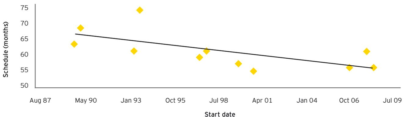
Figure 10 - Construction schedule for South Korean OPR1000<sup>20</sup>
