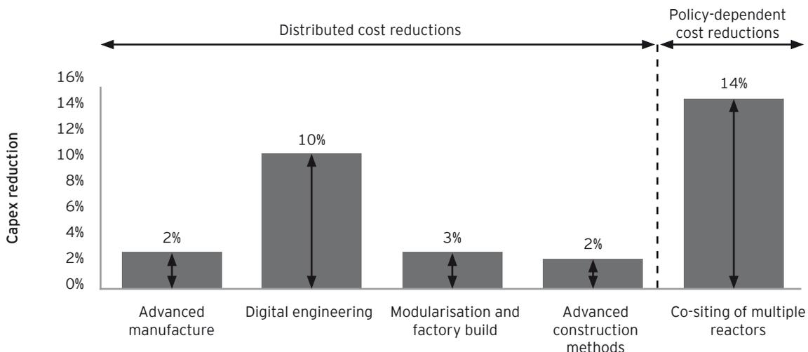
Figure 12 - The potential capex reduction through applying different techniques to SMR<sup>F</sup>
