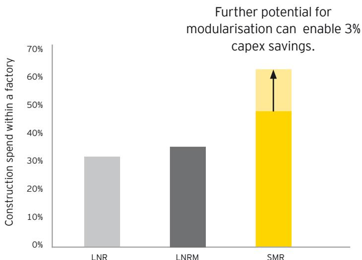
Figure 13 - Percentage of factory construction for different reactor types
