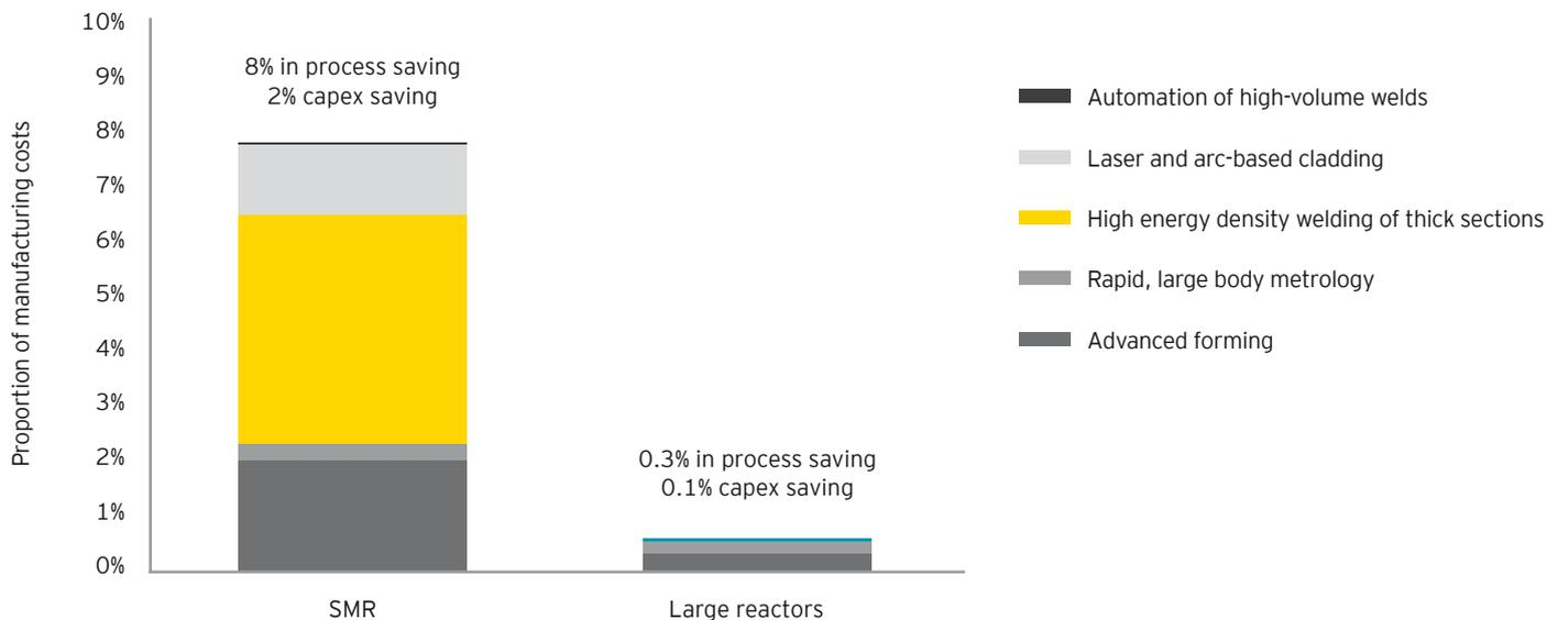
Figure 14 - The potential in-process savings through implementation of advanced manufacturing techniques<sup>H</sup>
