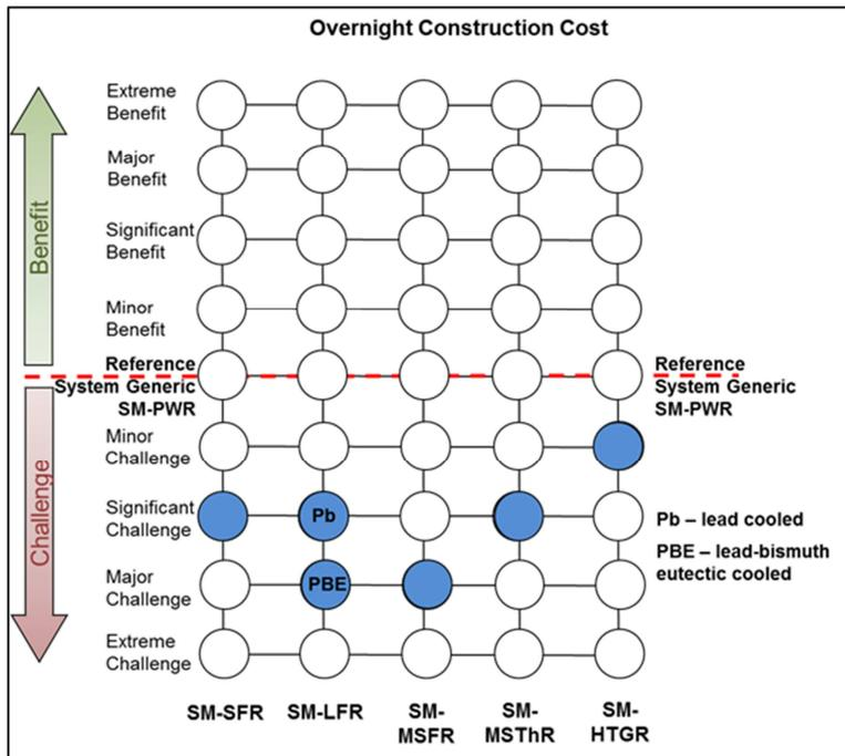
Figure 12: Overnight Construction Cost from GFAs
