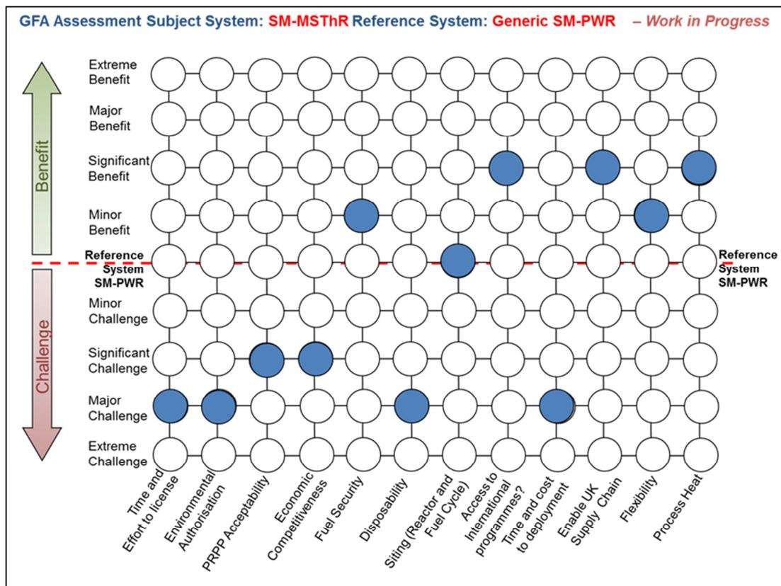
Figure 6: GFA of SM Molten Salt Thermal Reactor with Generic SM-PWR Reference
