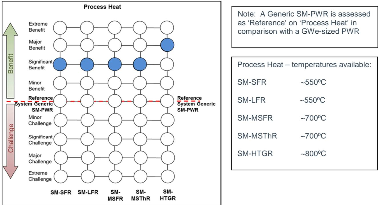
Figure 20: Process Heat from GFAs
