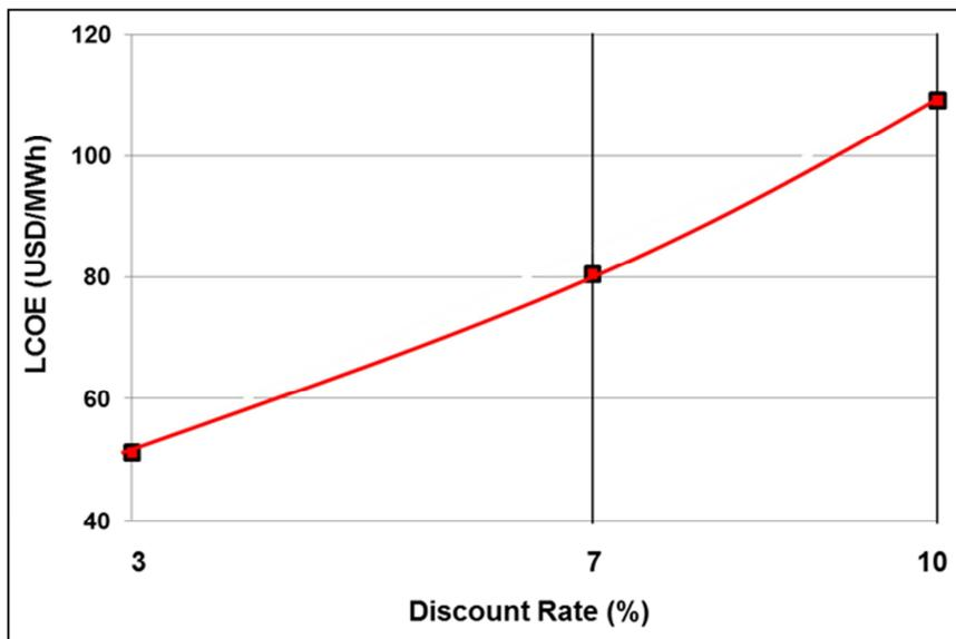
**Figure 22: Variation in LCOE with Discount Rate**
