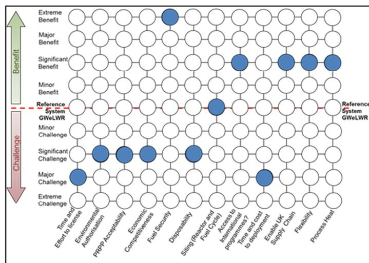
Figure 1: Comparison View for System Attributes compared to a Reference System (in this case a comparison of the Gen IV International Forum (GIF) Molten Salt Fast Reactor with a GWe-sized LWR) [5]
