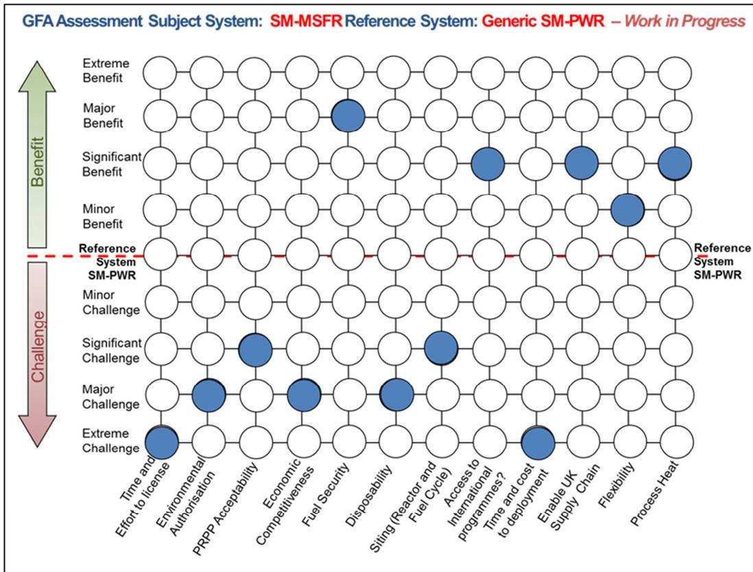
**Figure 5: GFA of SM Molten Salt Fast Reactor with Generic SM-PWR Reference**
