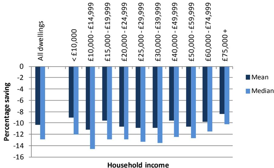
Figure 5.12 shows the distribution of percentage savings for properties having condensing boilers installed in 2007 and the comparator group. It shows that at all points in the distribution the properties that had condensing boilers installed in 2007 had a greater percentage reduction in consumption than the comparator group.
