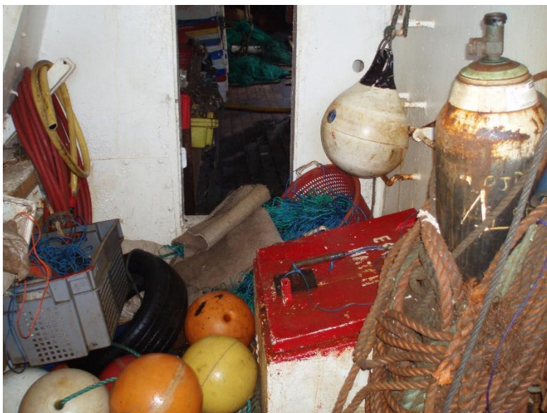
Risk assessing possible hazards - a cluttered store onboard a fishing vessel
