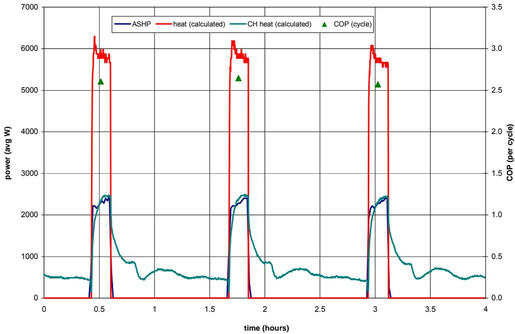
Average run time: 10.8 minutes    Cycle time ~ 75 minutes    max  $T_{flow} = 48.1^{\circ}C$
