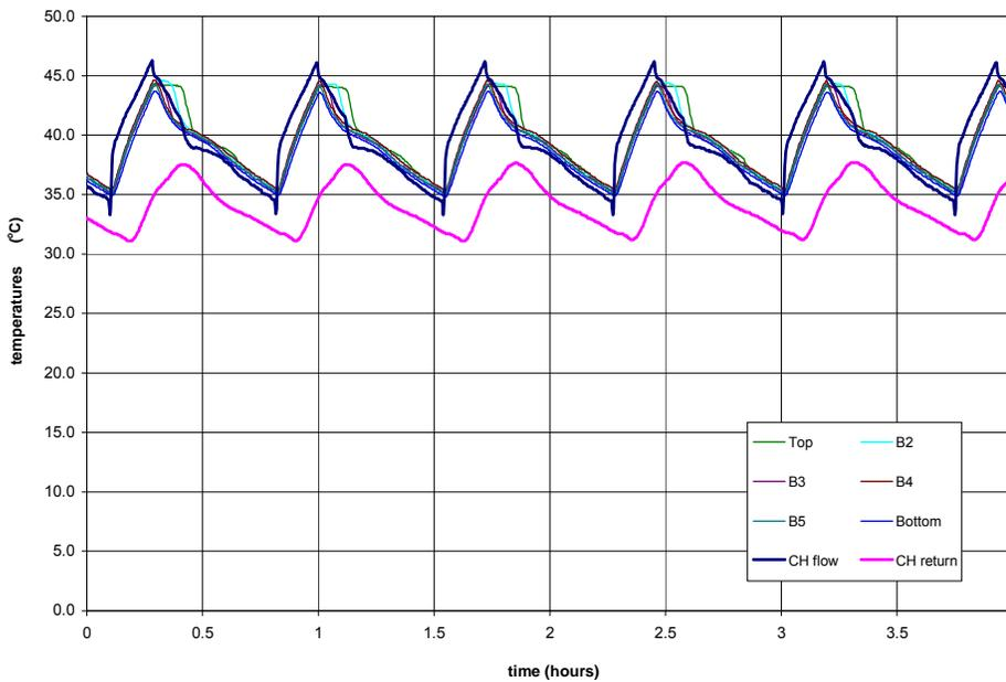
The cooling curve for the two radiator case is steeper (more radiator surface to dissipate the heat), although there seems to be less stratification of the tank.
