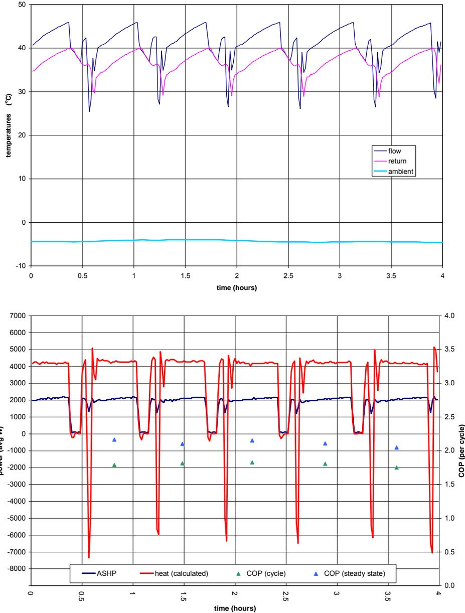
The “steady-state” COP is calculated for a 10 minute period towards the end of each run. The COP value for the complete cycle includes the defrost energy used.
