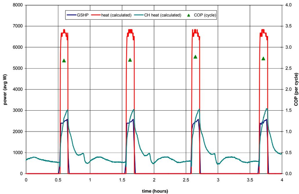
**Figure 5.1: Power (heat and electricity) and COP (forced cycling, 1 radiator)**
