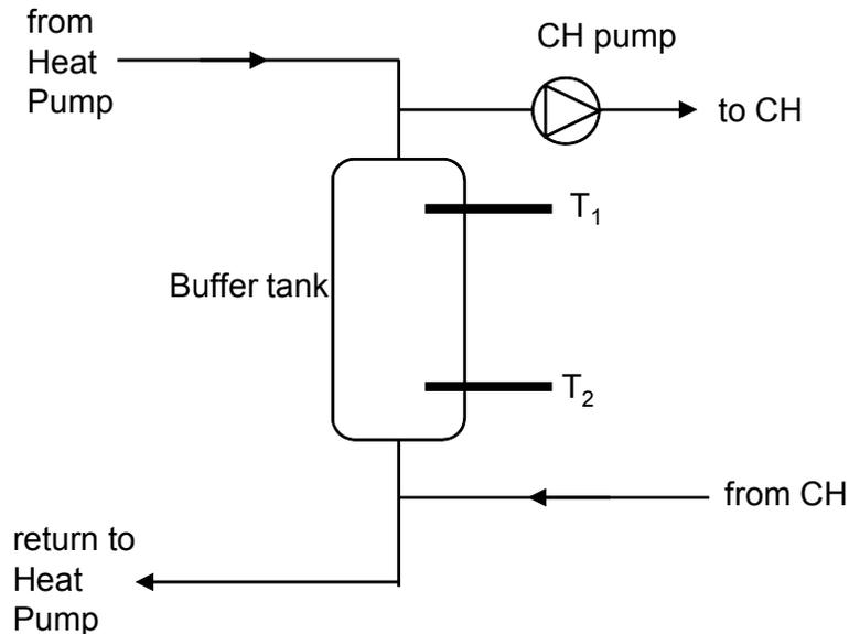
**Figure 4.1: Buffer tank set-up**
