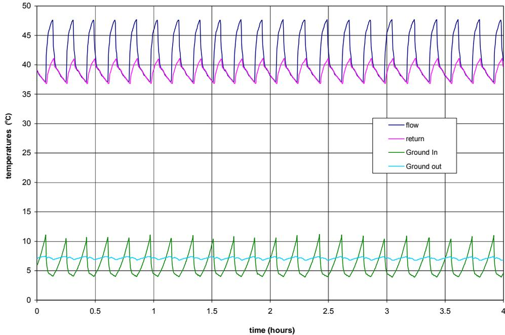
**Figure 3.2: Example temperatures under forced cycling conditions (3 radiators open)**
