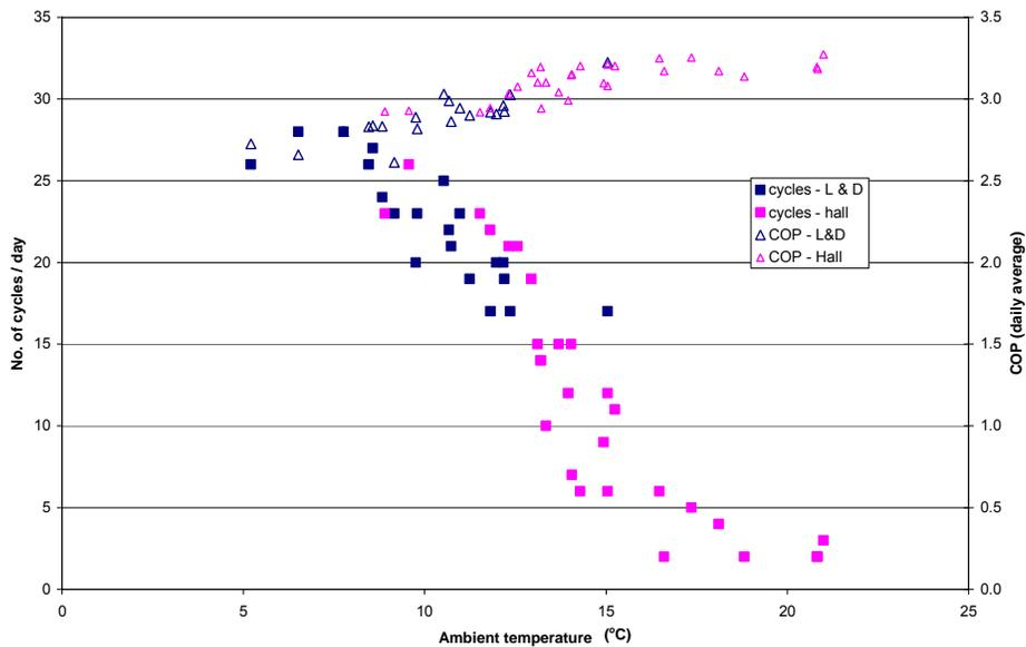
**Figure 6.4: Summary of ASHP and Buffer Tank in normal operation mode**
