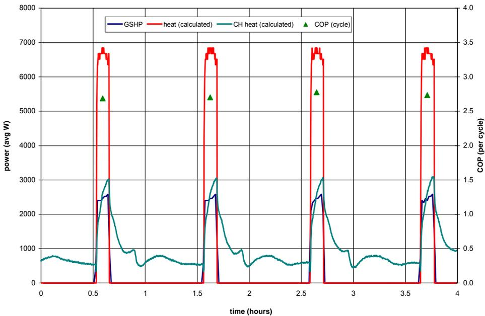
Average run time: 7.7 minutes    Cycle time ~ 62 minutes    max  $T_{flow} = 46.8^{\circ}C$
