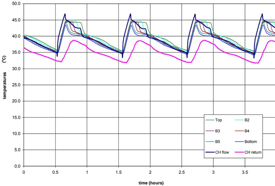
The buffer tank temperatures show some stratification after the heat pump switches off, but this is short lived and after around 20 minutes the tank cools as one mass.
