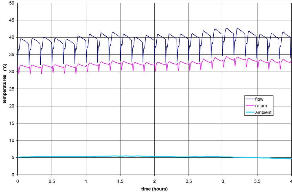
**Figure 2.4: Flow and return temperatures under room thermostat control (2 radiators)**
