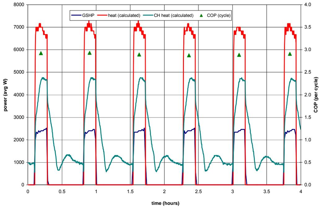
Average run time: 10.7 minutes    Cycle time ~ 44 minutes    max  $T_{flow} = 46^{\circ}C$
