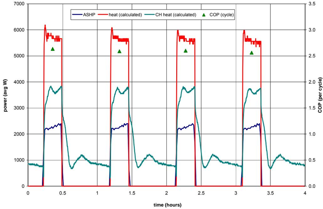
Average run time: 16 minutes      Cycle time ~ 57 minutes      max  $T_{flow} = 47.2^{\circ}C$
