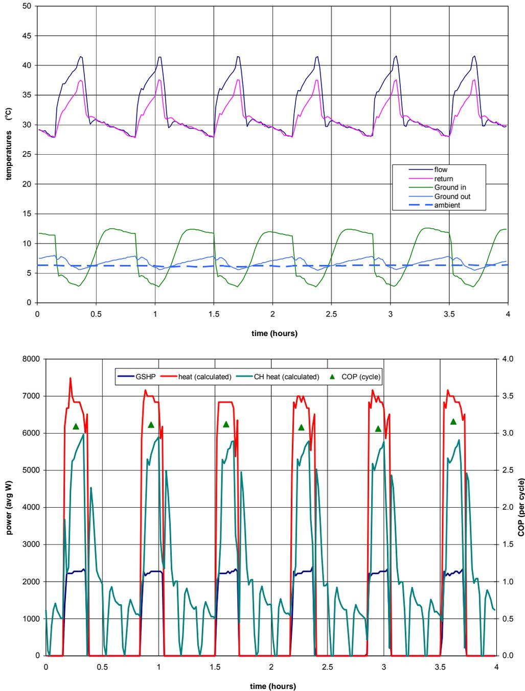
The lower graph shows the heat pump cycling regularly (blue and red lines). The Central Heating (the green line) cycles on and off during the heat pump off periods. This is due to the room thermostat being satisfied, and then calling for more heat.
