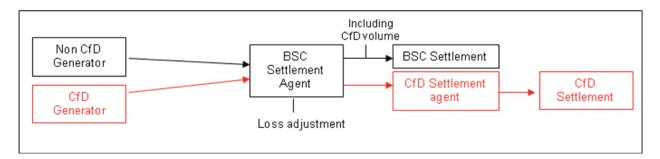
Figure 6: Illustration of measurement of output from generators registered as an additional BM Unit
