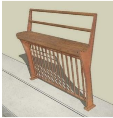
Option 2b: A corten steel railing with a wooden handrail and arm rest
