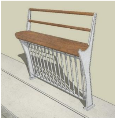
Option 2a: A galvanised steel railing with a wooden handrail and arm rest
