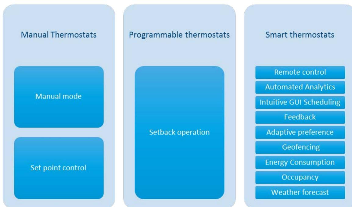
**Figure 5 Thermostat categorisation (adapted from Robinson *et al.*, 2016)**
