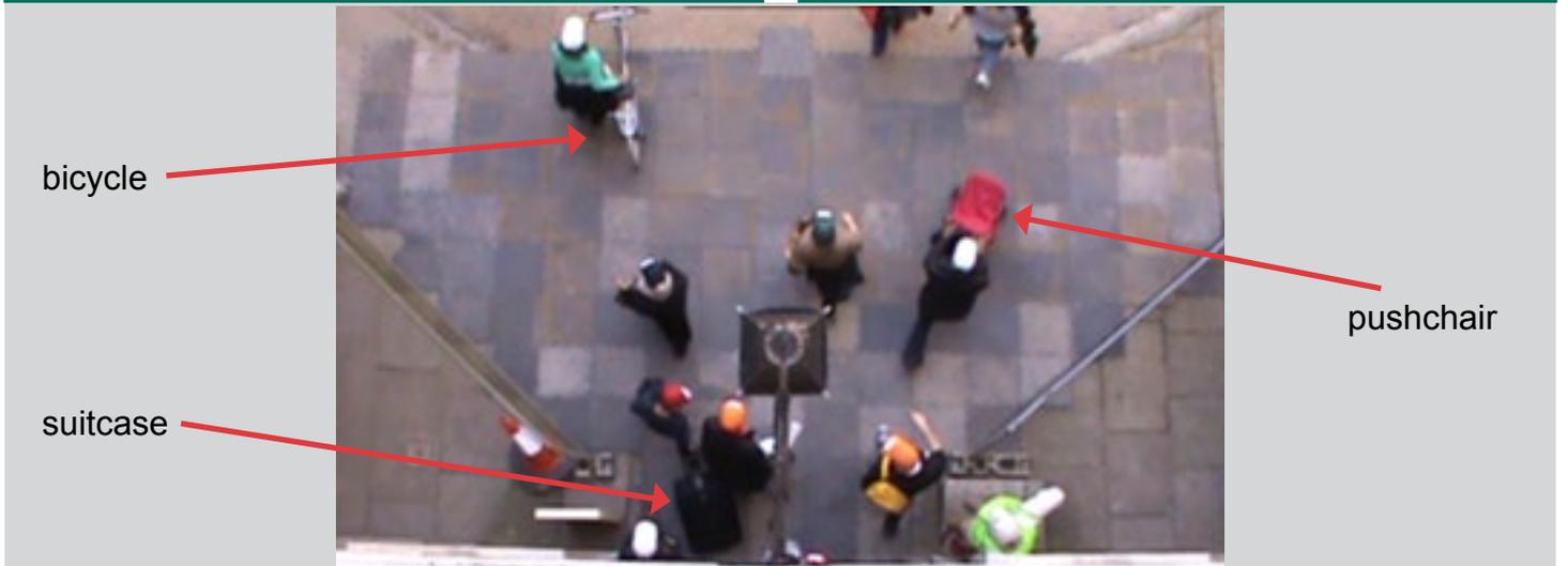
Figure 5: Experimental set-up, 2.4m exit width, without bollard array with 60% encumbrance level.
