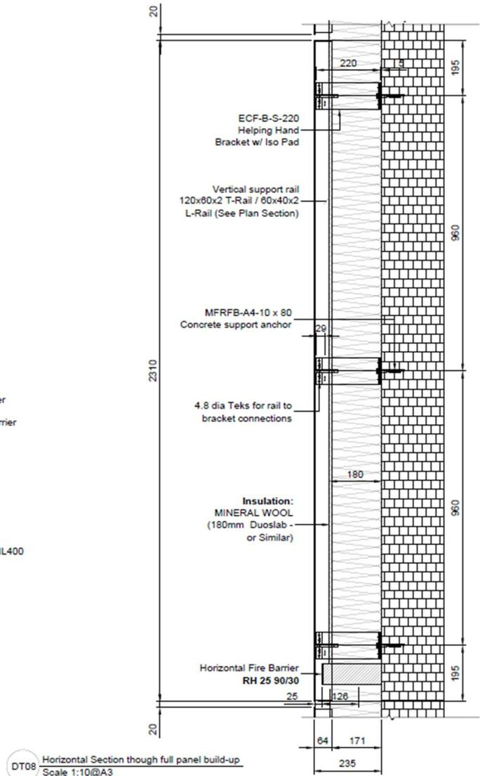
DT08 Horizontal Section through full panel build-up
