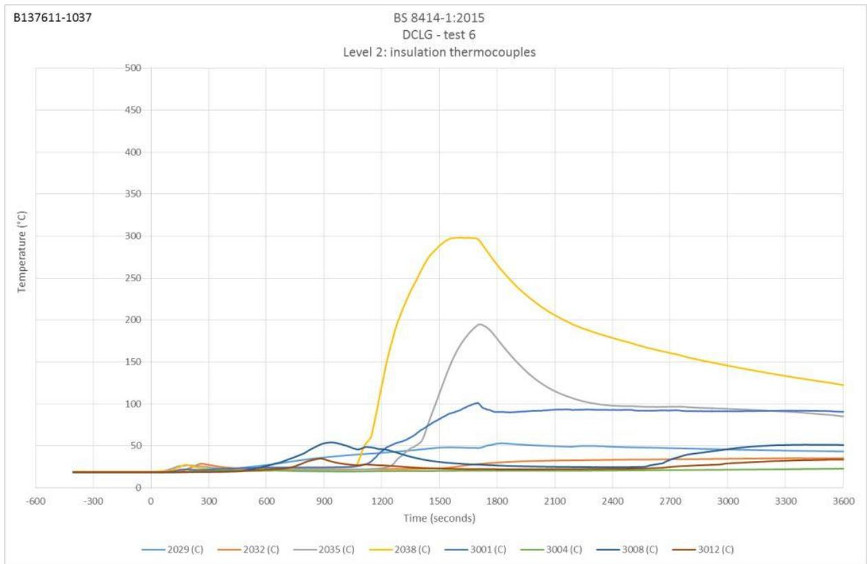
Figure 18. Level 2 insulation thermocouples.
