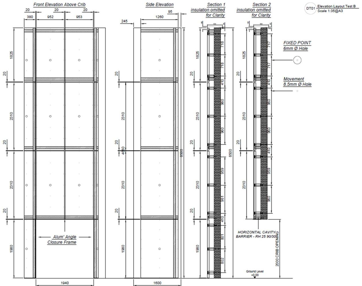
Figure 10. Front elevation, side elevation and vertical sections for the system (supplied by the Test Sponsor).
