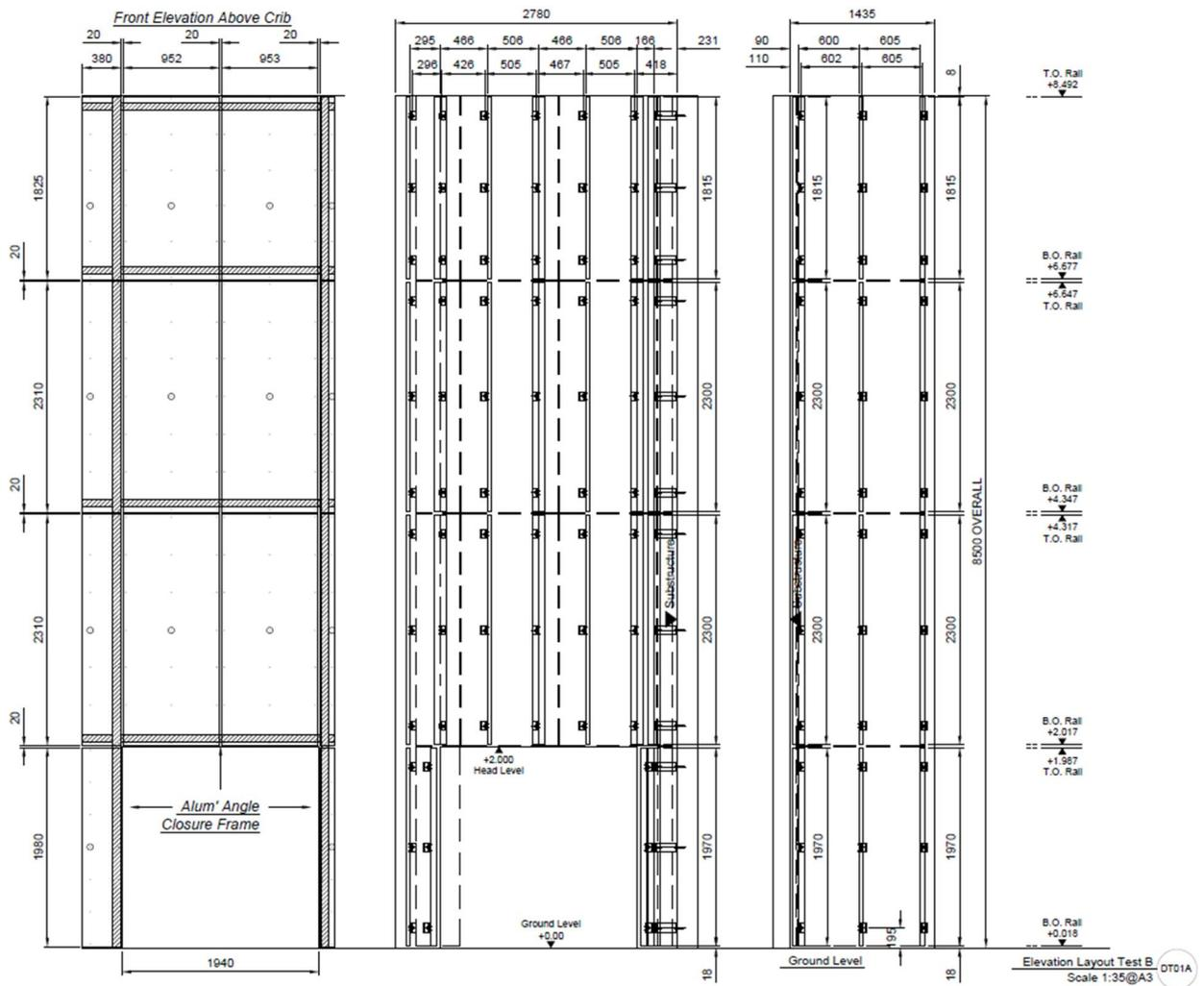
Figure 11. Front elevation, side elevation and vertical sections for the substructure system (supplied by the Test Sponsor).
