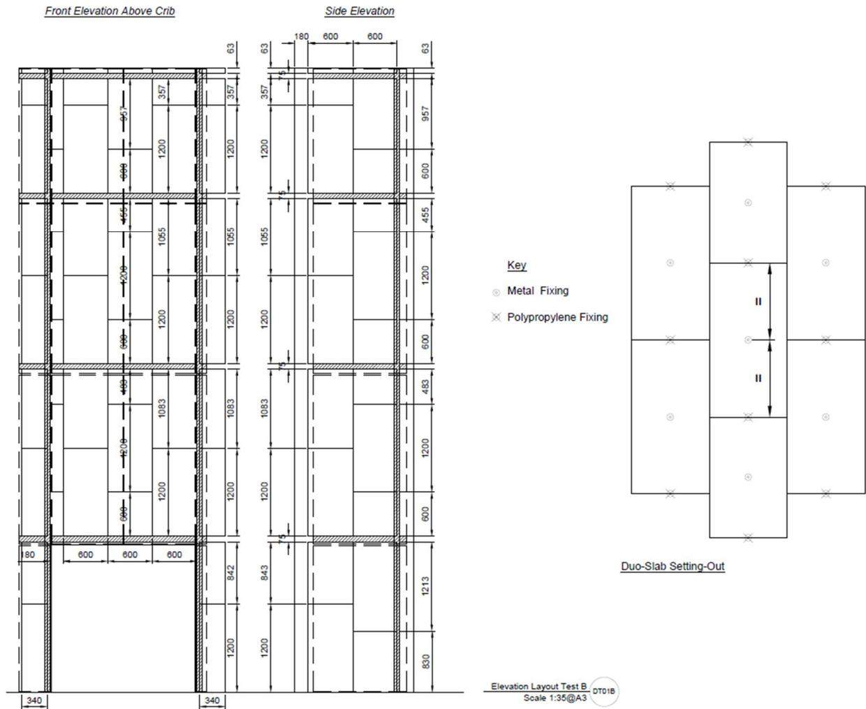
Figure 12. Front elevation, side elevation for the insulation panels installation (supplied by the Test Sponsor).
