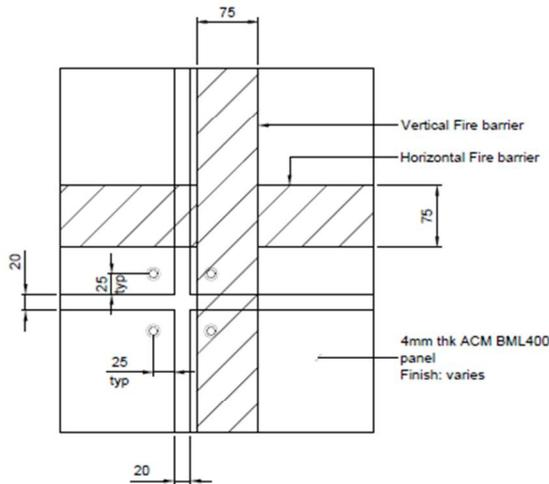
DT07 Enlarged detail on acm/fire barrier cruciform
