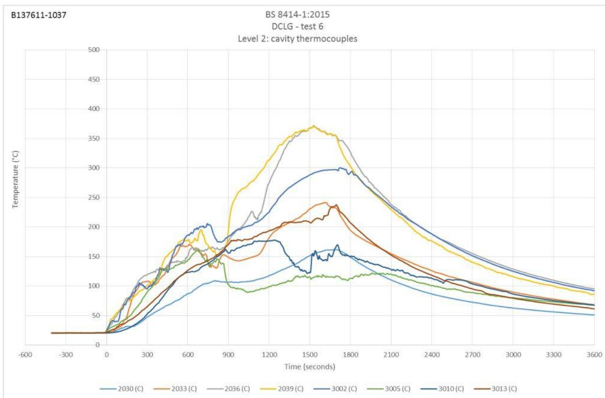
Figure 17. Level 2 cavity thermocouples.
