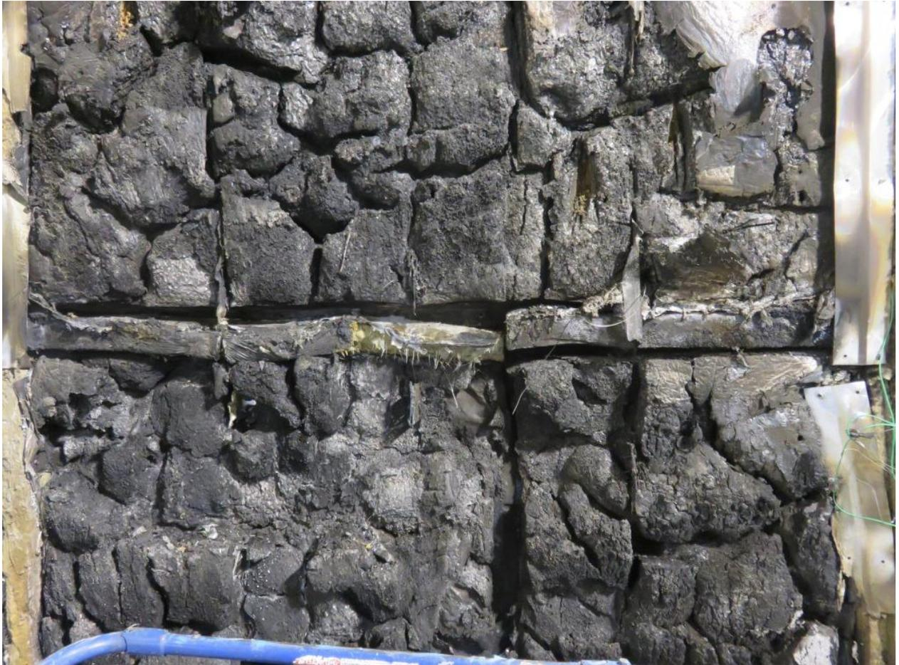
Figure 34. Close up of second cavity barrier in line with the combustion chamber opening.
