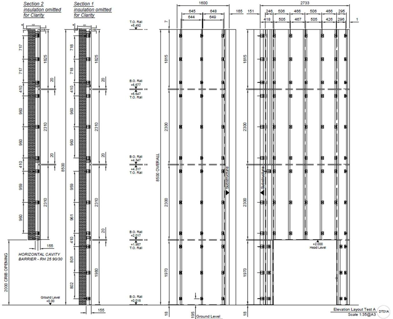
Figure 14. Front elevation, side elevation and vertical sections for the substructure system (supplied by the Test Sponsor).
