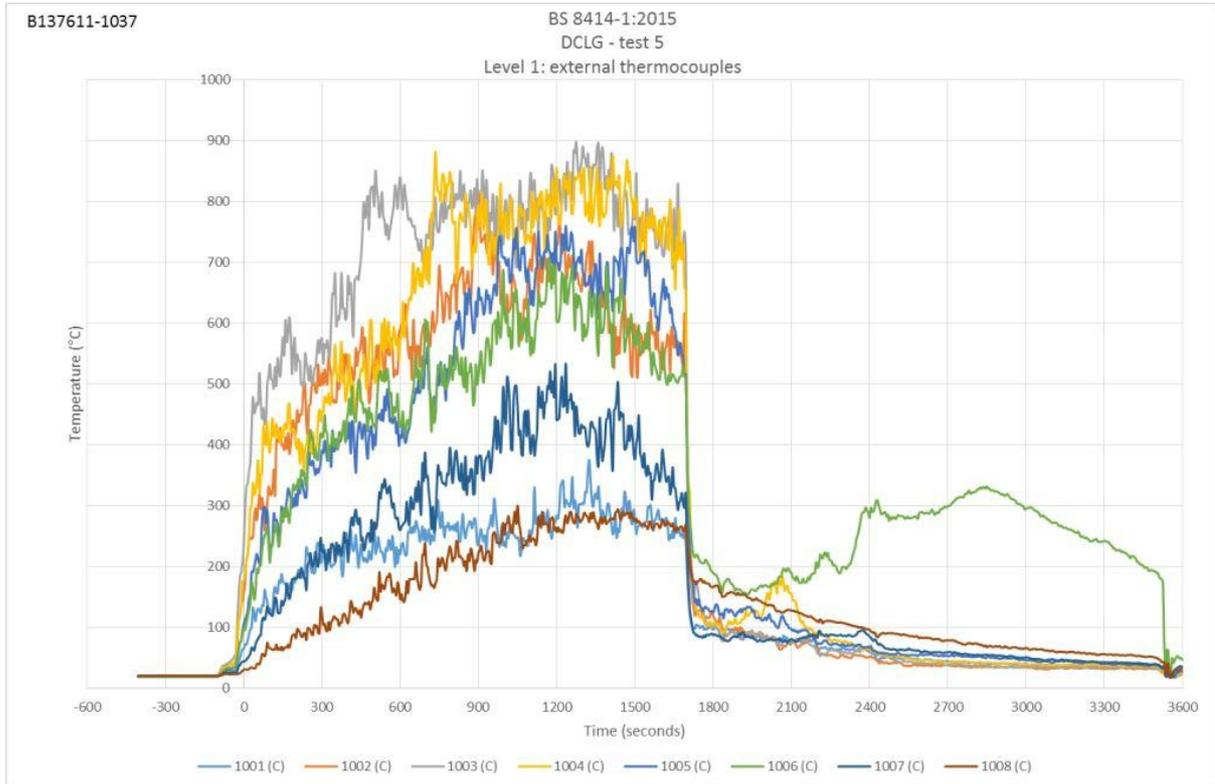
Figure 18. Level 1 external thermocouples.
