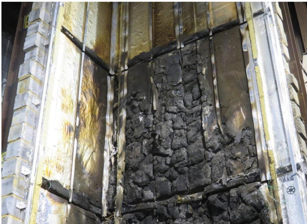
Figure 32. Damage to cladding system beneath ACM panels between the second and third horizontal cavity barrier (approximately 2400-4700mm above combustion chamber).
