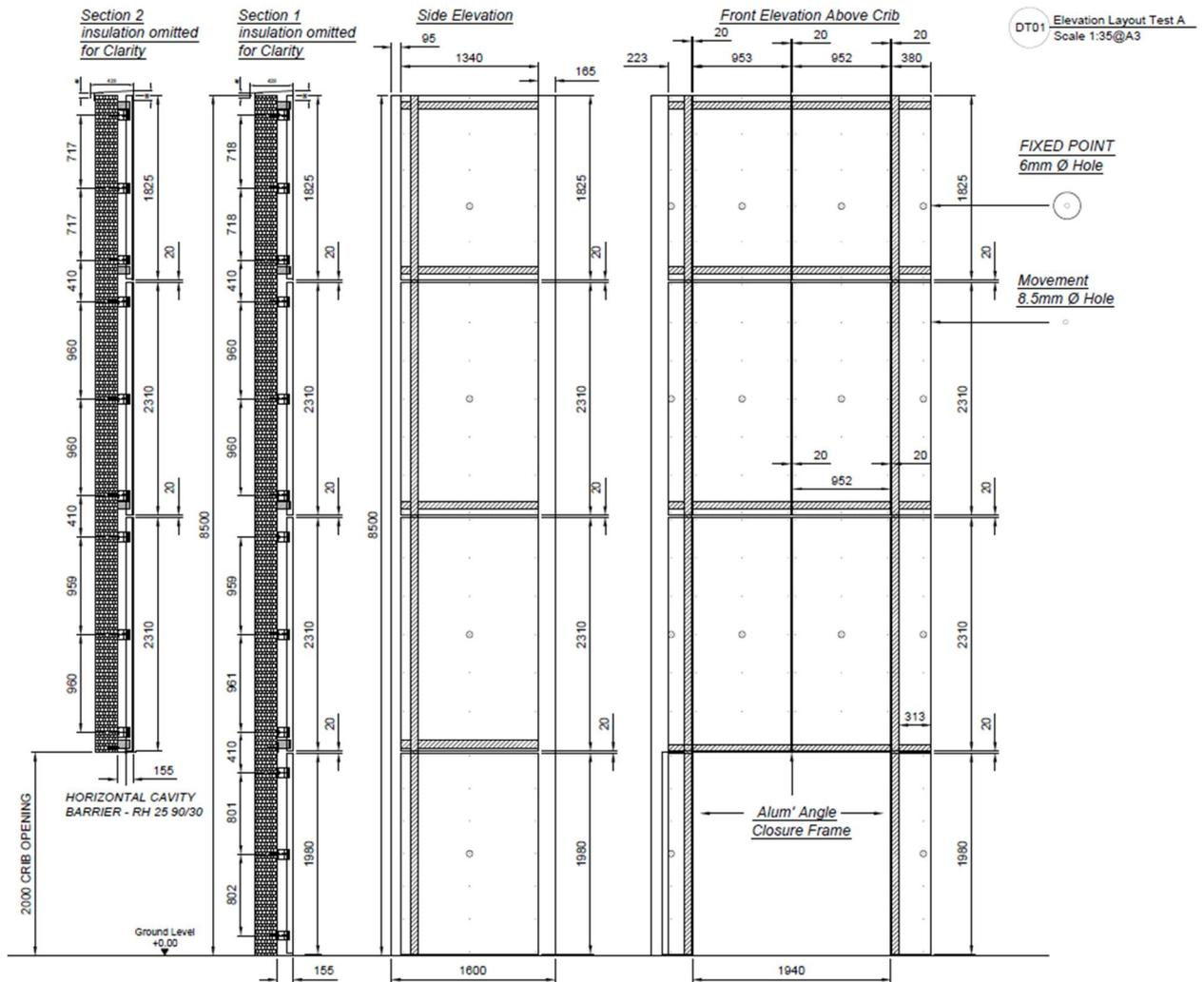
Figure 13. Front elevation, side elevation and vertical sections for the system (supplied by the Test Sponsor)
