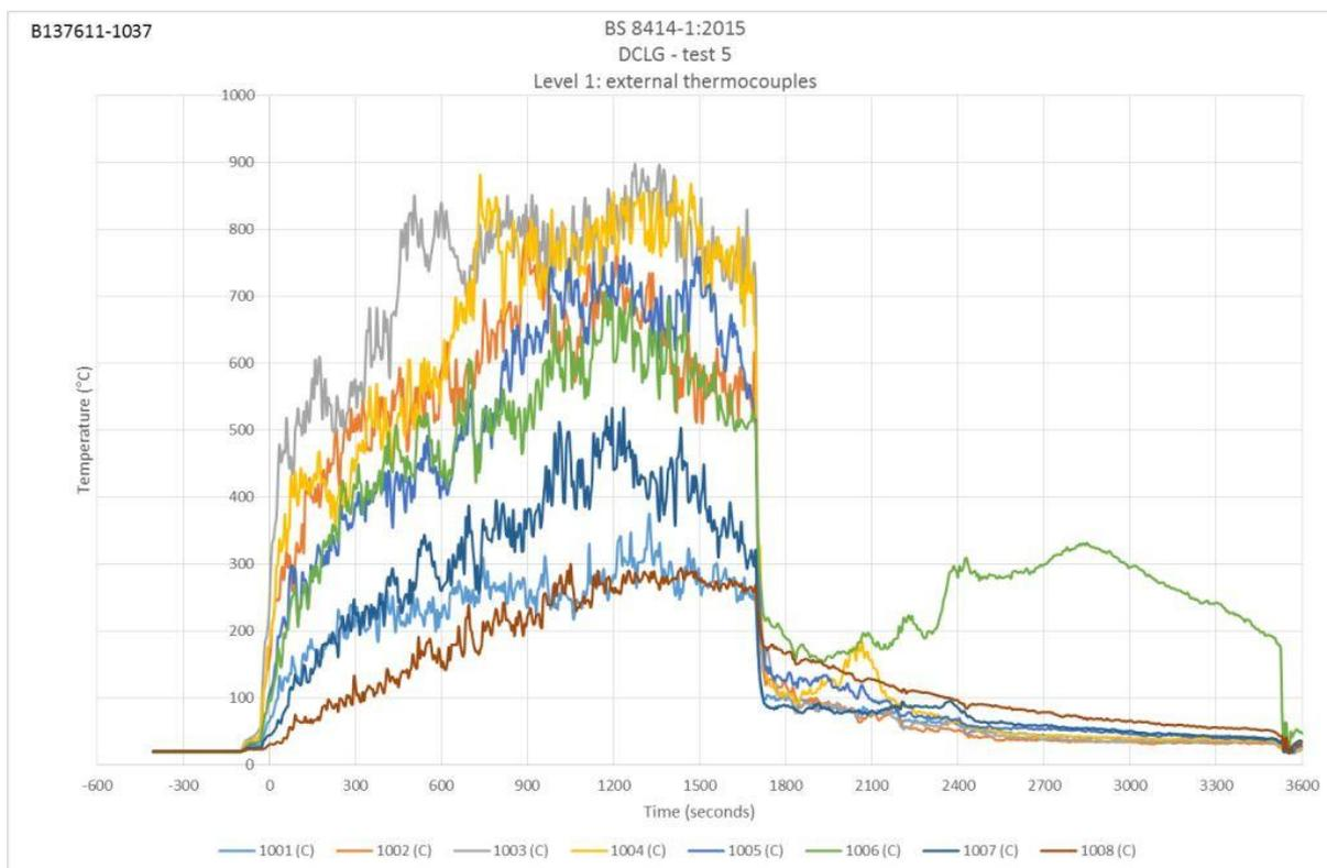
Figure 18. Level 1 external thermocouples.
