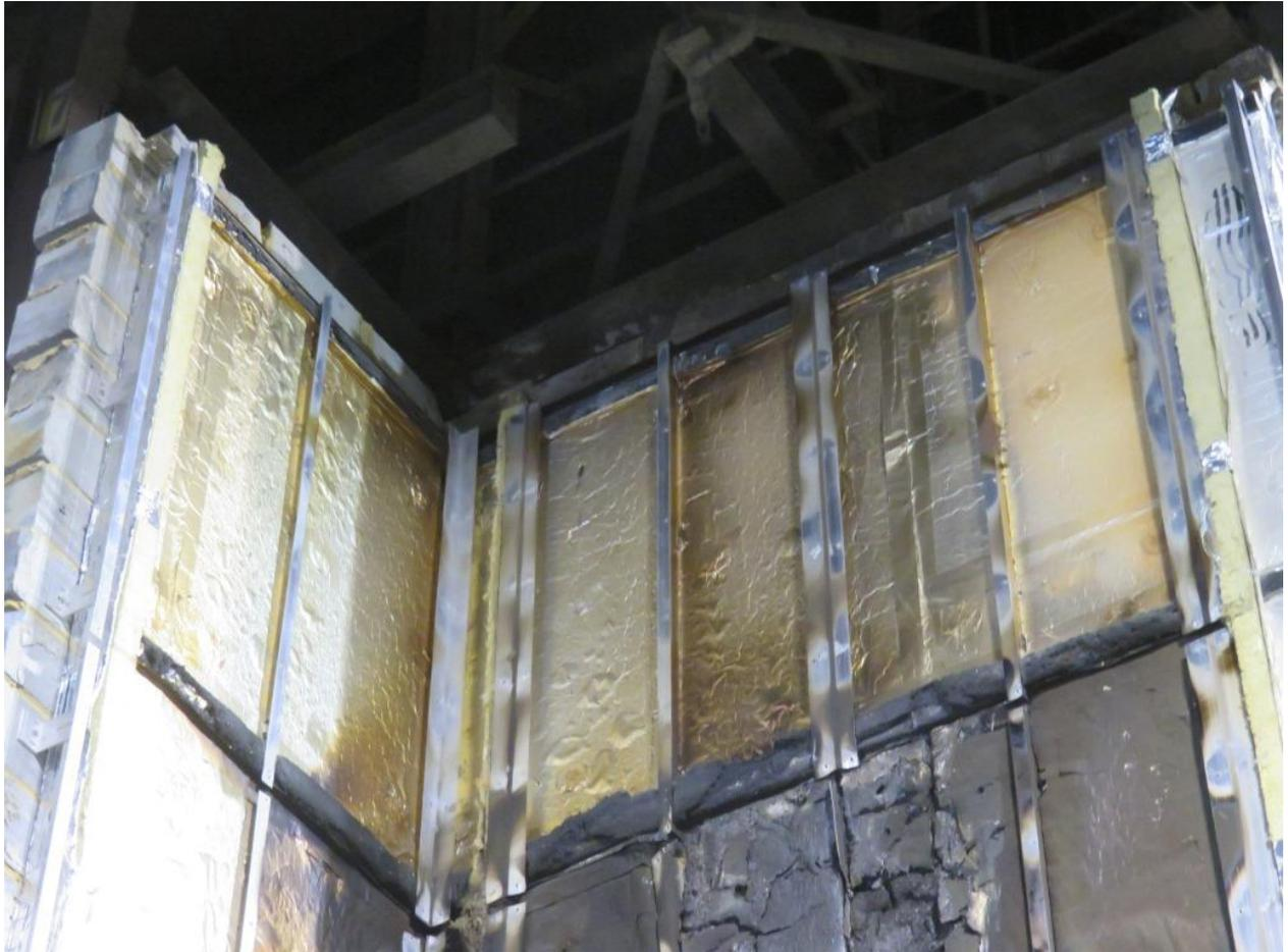
Figure 33. Damage to cladding system beneath ACM panels between the third and fourth horizontal cavity barrier (approximately 4700-6400mm above the combustion chamber).
