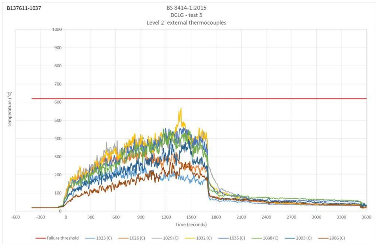
Figure 19. Level 2 external thermocouples.
