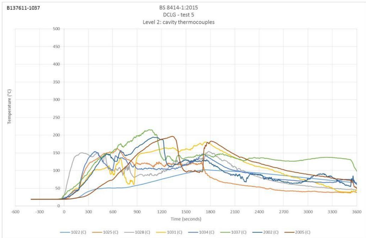
Figure 20. Level 2 cavity thermocouples.
