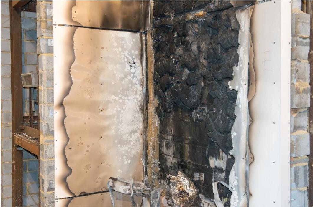
Figure 25. First row ACM panels (directly above combustion chamber).
