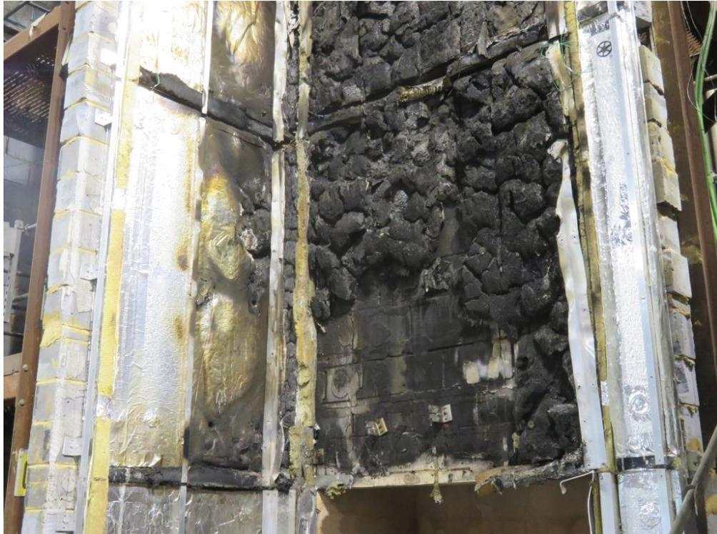
Figure 31. Damage to cladding system beneath ACM panels directly above combustion chamber.
