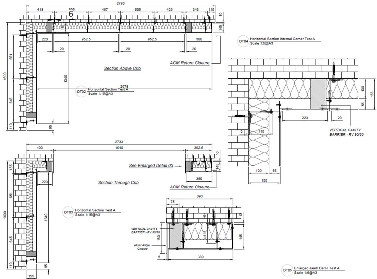
Figure 16. Horizontal section through and above the combustion chamber, and installation details for the system (supplied by the Test Sponsor).
