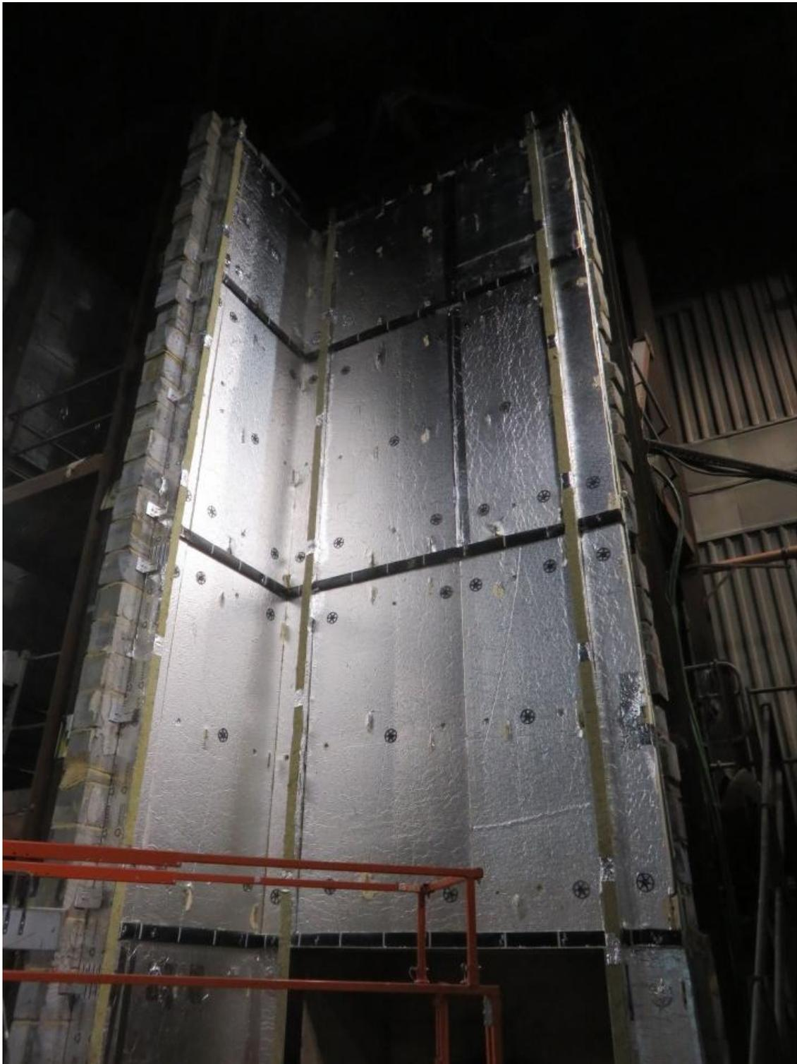
Figure 7. Installed cavity barriers and PIR insulation panels.
