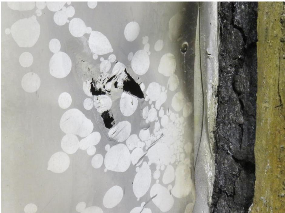
Figure 26. Close up view of partial panel consumption on the wing wall.
