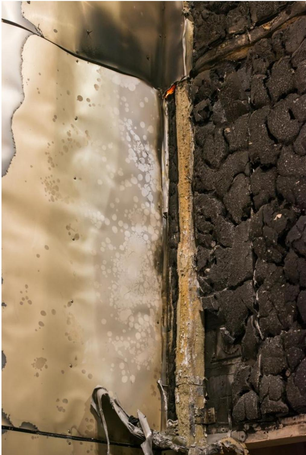
Figure 35. Close up of vertical cavity barrier adjacent to the wing wall directly above the combustion chamber (photograph taken during the 30-60 minute test period).
