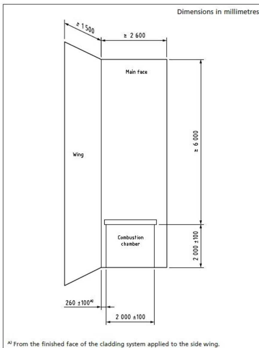
Schematic 1. Test apparatus dimensions as specified by test Standard<sup>[1]</sup>.
