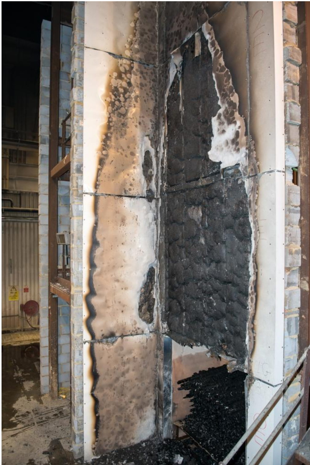
Figure 25. Full height photograph of system after test termination – wing wall.
