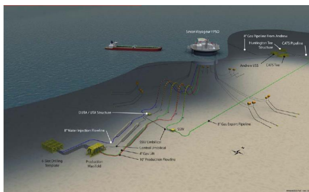
Figure 2.10 – Schematic layout of the Huntington field
