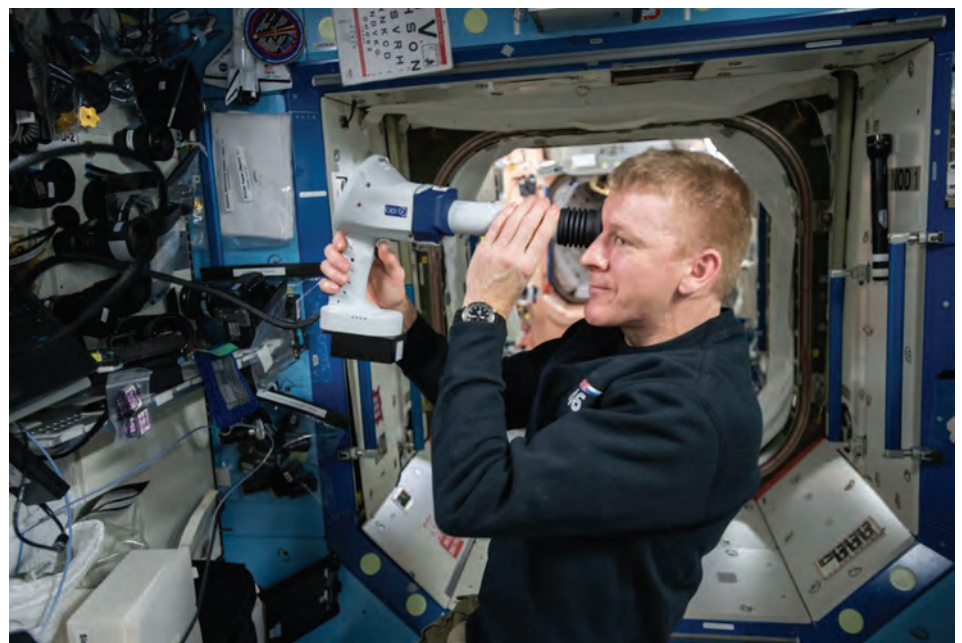
This device is used to capture images of blood vessels in the eye as part of studies of eye health in astronauts Credit: ESA, NASA
